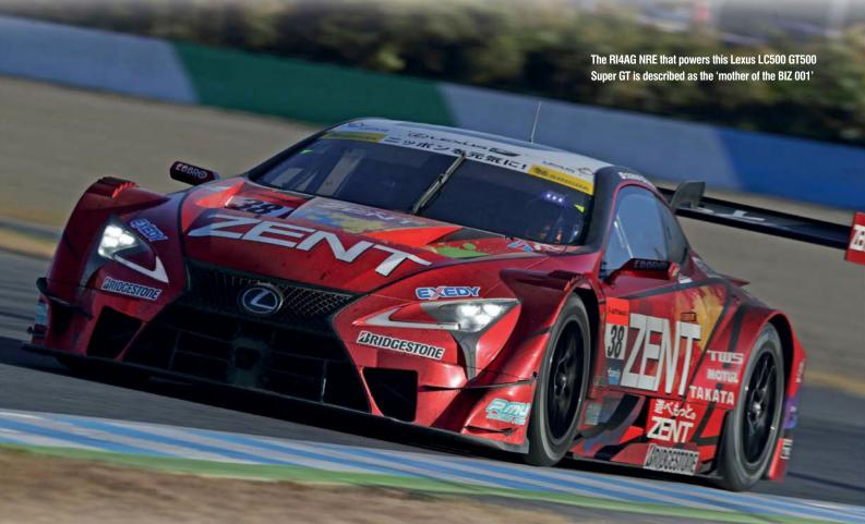
season both of Japan's top racing categories, namely the GT500 class of Super GT and the open wheel Super Formula championship, adopted a brand new engine formula. Dubbed NRE (Nippon Race Engine) the new regulations mandated a 2-litre turbocharged in-line 4-cylinder design featuring direct injection. As was the case with Formula 1 and LMP1, the rules also saw the introduction of a fuel flow limit, although in this case governed
