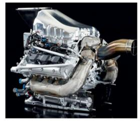
In 2014 and 2015 Mercedes and Honda (pictured) used exhaust layouts designed to allow the MGU-H to recover maximum energy. The new regulations should switch focus on to maximising the ICE
