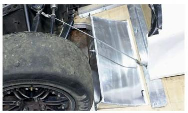
The Aries team fabricated these adjustable diffusers. Lock-nut arrangement (centre) allowed the front diffuser ramps, hinged below with tape at the transition, to be adjusted for angle
