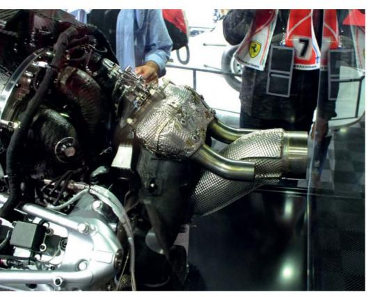
Attempts to improve the sound of the current F1 power units has seen separate wastegate exit solutions tried, but with little effect. Upping the maximum revs by 3000rpm to 18,000rpm is the approach being looked at for the 2021 PU regulations
