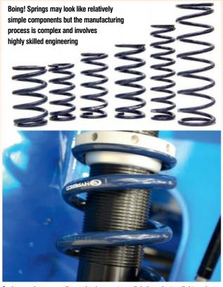
Spring perches on a coilover shock are not parallel; they sit at a slight angle
