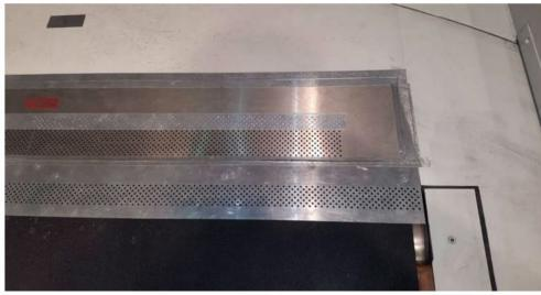
Middle and above: The Boundary Layer Removal System (BLRS) is made up of a primary and then secondary perforated suction plate. The secondary plate sits on the moving belt and is of high-grade aerospace aluminium to prevent it buckling
