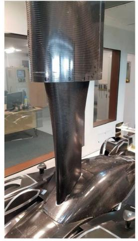
The wind tunnel model is attached to a carbon support strut that is connected to a six-component pyramidal virtual centre balance
