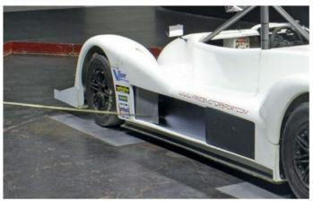
Silver-taped wheel fairings can be seen behind the front wheels; the results were better without these in place. Sidepod undercuts are just above the running boards
