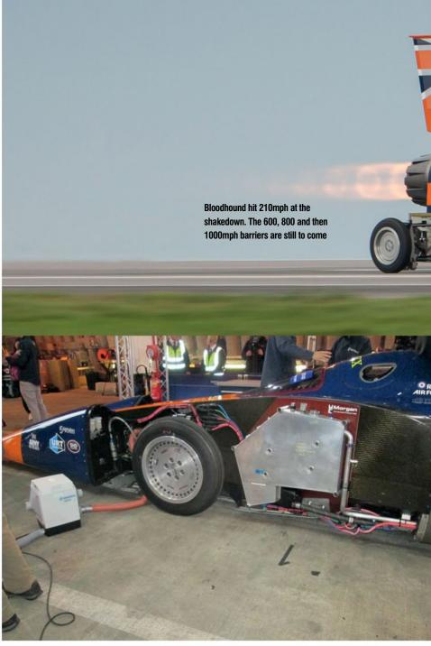
Minor brake fire was the only problem. Braking will involve air brakes, wheel brakes and two parachutes
