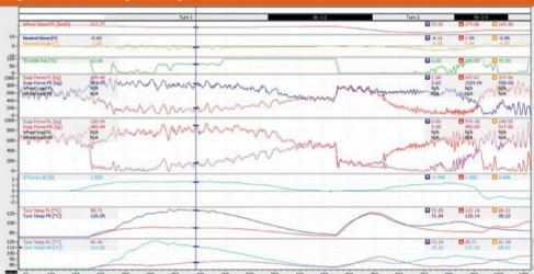
The tyre temperature model in ChassisSim can help to show how the tyre gets up to its working temperature in the first place
