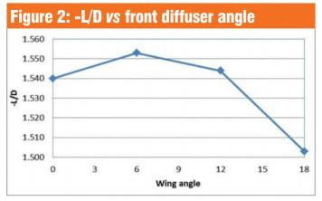
Figure 2: The aero efficiency appeared to peak at the 6-degree front diffuser angle
