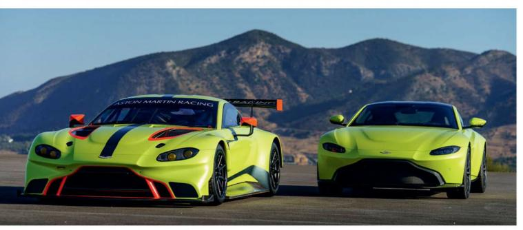
The Vantage GTE alongside its road car cousin. AMR benefited from access to the standard car on the prototype line and was able to specify some race components very early on
