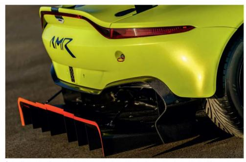
Carbon fibre and steel five-piece floor features splitter, three mid-car sections, and runs into a whopping diffuser at the rear
