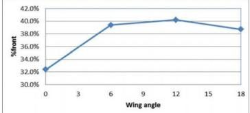
Figure 1: This shows that % front appeared to peak at the 12-degree front diffuser angle
