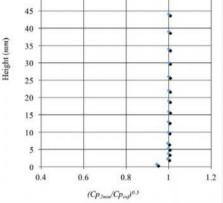
take long for the boundary layer to re-grow as shown in **Figure3**, where the thickness has increased to around 10mm and is removed again by the secondary suction plate (**Figure4**). When the flow reaches the moving belt, the flow is energised, again, reducing boundary layer growth, achieving a thickness of approximately 0.5mm (**Figure 5**) before the air reaches, and interacts with, the car.
