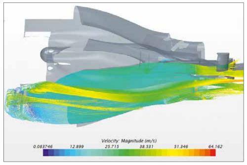
Airflow under the body and through sidepods was calculated in CFD to ensure adequate flow and a good level of efficiency
