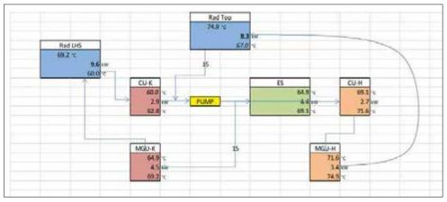
Figure 7: The single pump would have been workable but the demands of the oil system and ERS cooling counted against it
