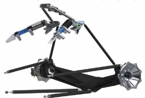
In addition to hydraulic interconnected suspension Edith Cowan's car features a beam axle and a heave spring at the rear
