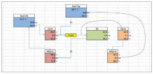
Figure 4: In first ERS cooling circuit devised by Caterham the small central cooler would feed the control unit for the MGU-K
