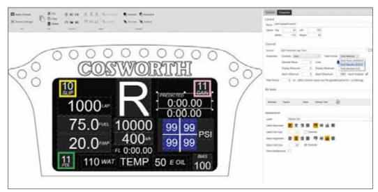
The display has an overlay feature which allows the driver to show only the relevant data at any appropriate time
