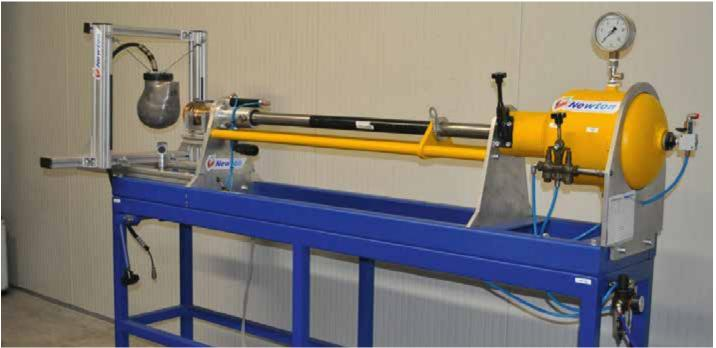
The projectile is loaded into the barrel of a pneumatic gun powered by a pre-charged reservoir of compressed air (this test rig was developed by the FIA and Newton Laboratories)
