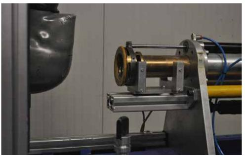
The velocity of the projectile is measured at the muzzle of the gun. The target is instrumented with a tri-axial accelerometer
