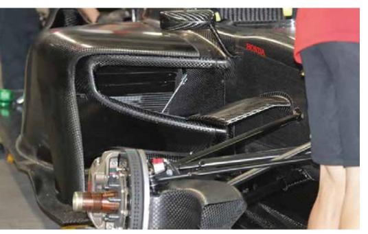
The Formula 1-style chassis wing drives air into the radiators while it also has a secondary function of increasing downforce
