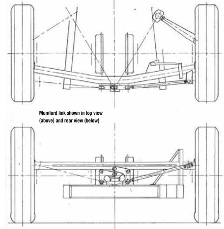
through the stock bump stop frame, which I have shown only on the right side; the left side has a mirror image one as well. These frames bolt to the main frame rails, so they can be slipped down over the De Dion tube.
