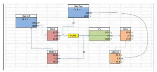
Figure 5: Team looked at integrating energy store cooling into the MGU-H circuit and making greater use of centreline cooler
