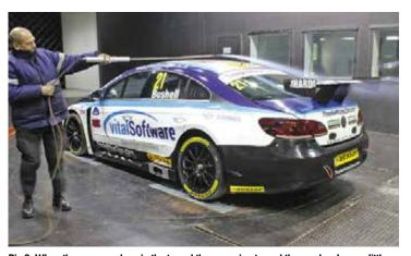
Pic 3: When the car was alone in the tunnel the rear wing turned the smoke plume a little
