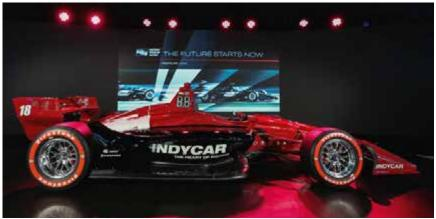
Launch of the UAK18 aero kit. Aesthetics were a major design consideration and this is the first IndyCar since 2007 to run without an airbox. IndyCar is also looking at a screen rather than a Halo for its cockpit protection
