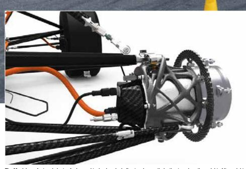
The Munich car featured plenty of advanced technology including topology optimisation to reduce the weight of its upright. It also made use of GKN metal additive manufacturing techniques to minimise the motor housing so to fit within the wheel hub
