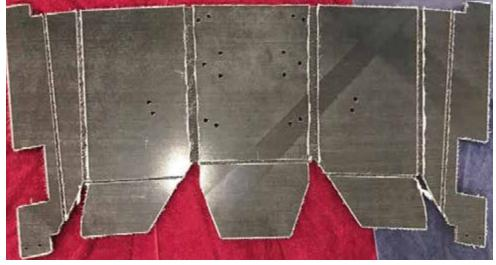
Cut and fold is a cheaper alternative to making moulds and doing a full composite layup. This is Edith Cowan's pattern for its monocoque. Note where the carbon fibre skins and the honeycomb have been CNC routed to allow the material to bend
