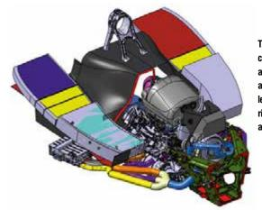
The final Caterham CT06 cooler layout. Two charge air coolers with ERS and oil and water coolers are on the left side, water cooler on the right. The gearbox cooler is above the turbocharger
