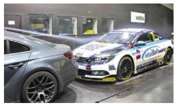
Pic 2: The lack of a rear wing on the leading car produced a very different flow field
