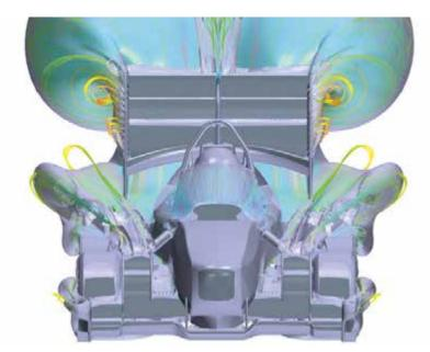
The Munich car features a very advanced aerodynamic package including DRS on the rear wing, a Formula 1-style shark fin, a monkey seat and a complex front wing and undertray
