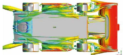
As well as spending 20 hours in the wind tunnel Monash also ran around 400 CFD simulations during development. Here we can see the Q-Criterion isosurfaces in Ansys, showing the vortices with the colour representing coefficient of total pressure
