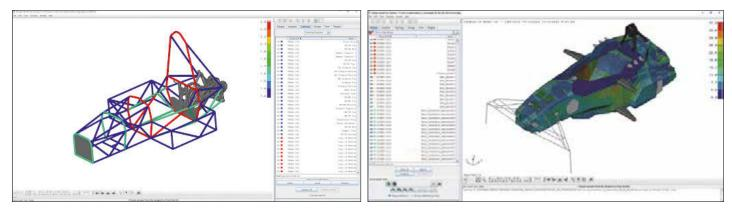
Steel spaceframes, such as this design from Warwick Racing in GRM Genesis software (left), are an effective solution for Formula Student. Full moulded monocoques, such as this Formula 1 example (right), are lightweight and have increased torsional stiffness. It is often the expense of the latter approach that drives Formula Student teams to opt for the former
