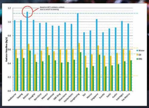
Figure 1: The first step was to map out the expected cooling demands over a season, including the extreme temperatures
