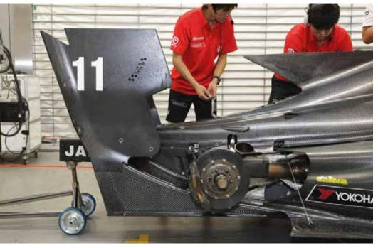
The aero work has been focussed on overtaking. At the rear of the car one of the carry-over parts from SF14 is the gearbox
