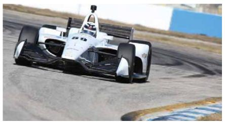
Road course kit being put through its paces in testing. The new aero has lessened the loads which means the more powerful engines can be introduced without too much concern about the suspension and tyres coping
