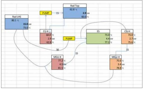
Figure 6: A second pump was added to serve the CU-K and this was to be fed via a cooler on the centreline of the racecar
