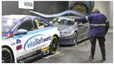
Pic 1: A closely following car modified the aerodynamics of the leading car, and vice versa
