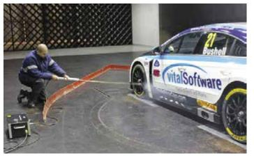
Boundary layer trip fence (the red strip above) had to be removed to fit a second car in
