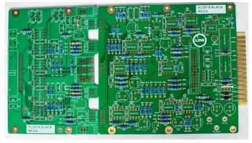
After Placing and Soldering all Resistors, we solder the next bigger parts like IC-Sockets and small Capacitors, like 37x100nF and 16x22pF
