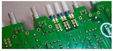
Check the alignment of the switches and pots from the upside again and try to bring them in line like the silkscreen is printed. After that install the blank bracket on the upper subboard and solder the pots in place.
