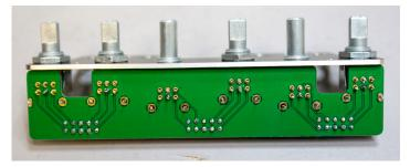
After having one pin of each pot soldered we add the bracket ike shown in the picture above. The direction of the bracket is shown in the picture below. After having all pots screwed to the bracket, we can solder all pins, then we need to cut the pins.
