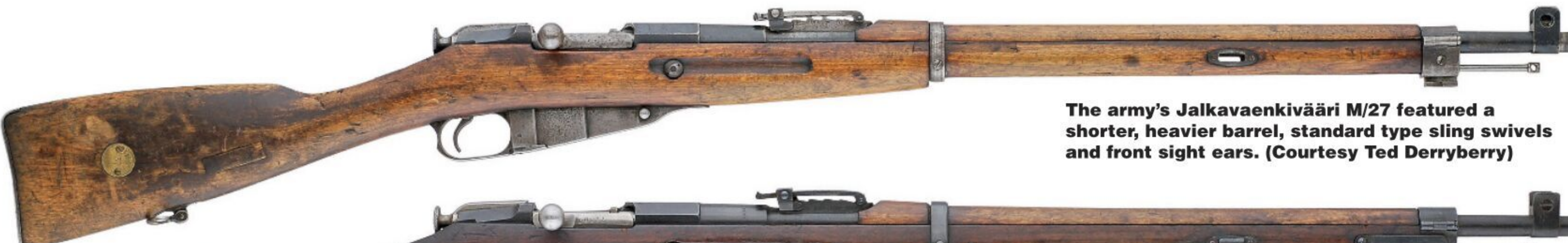
Late production M/27s had a reinforced barrel/bayonet band. (Courtesy Ted Derryberry)
