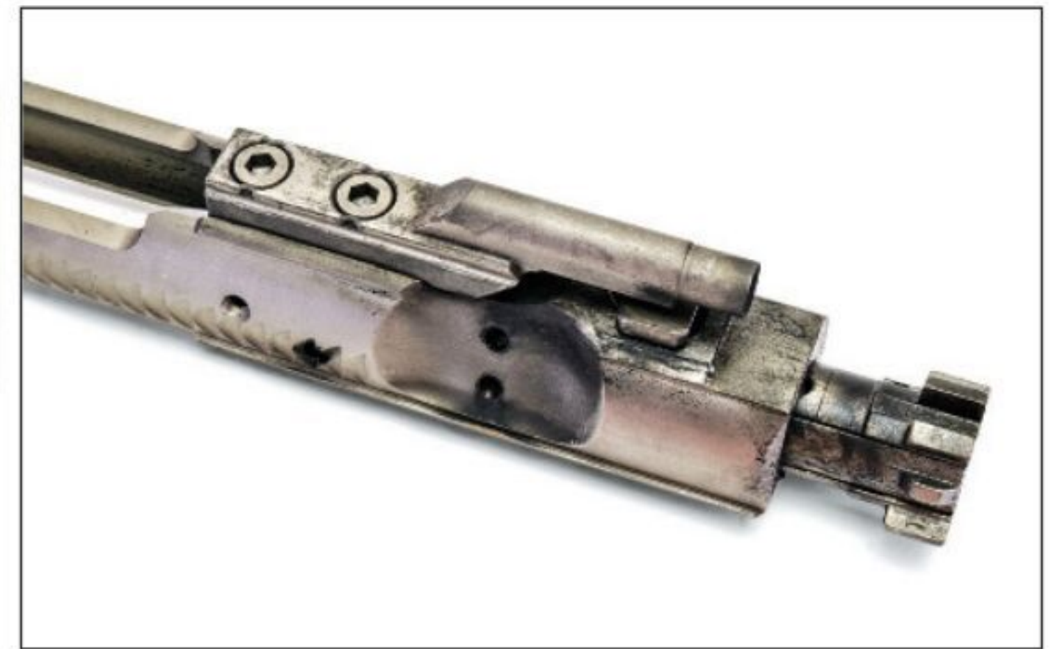
The nickel boron coating on the bolt/carrier keeps it slick, which helps to keep it running longer when its dirty. It is far easier to clean than a standard bolt carrier.
