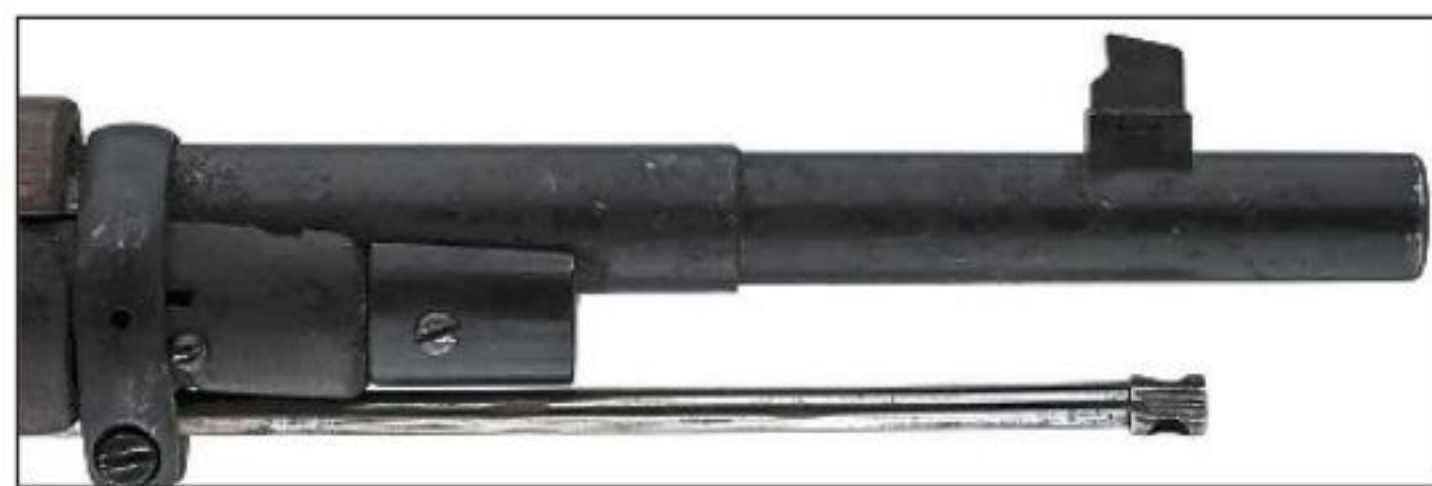
Jalkavaenkivääri M/91-24’s muzzle was reduced to allow mounting the obr. 1891g socket bayonet. (Courtesy Ted Derryberry)
