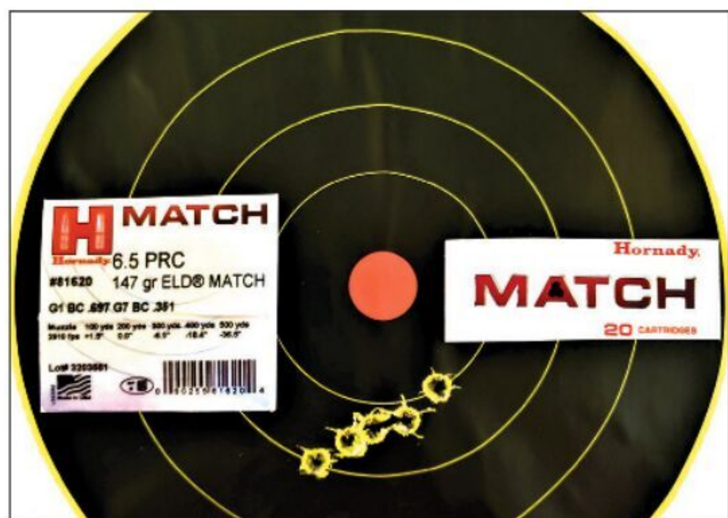
It's a tie! The Hornady 143-grain ELD-X Hunter and 147-grain ELD Match scored twin 1 1/2 inch groups at 200 yards.
