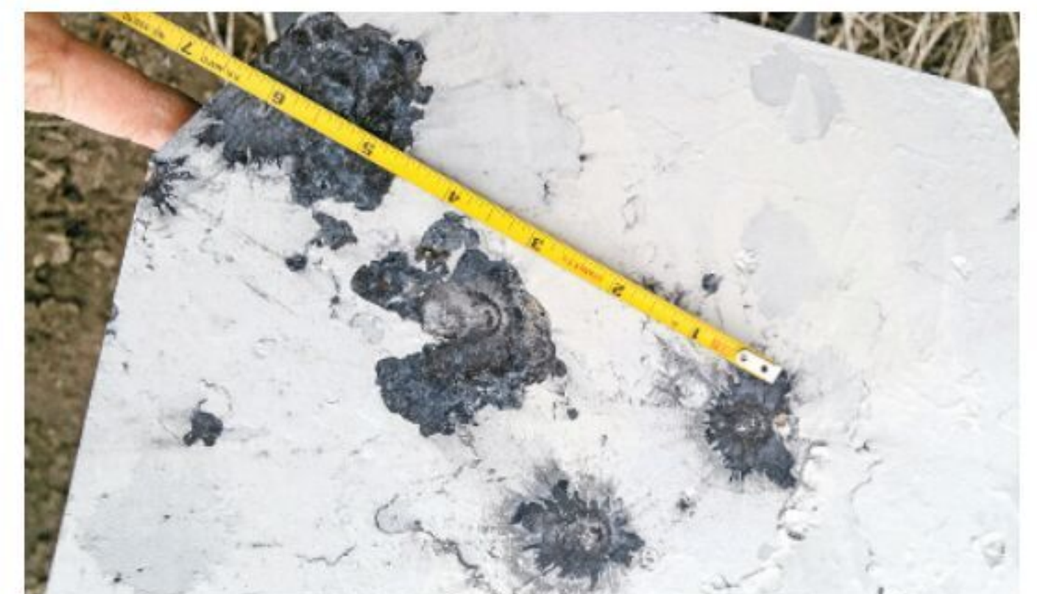
This 800-yard group has three rounds in 3.5 inches and all five in 6 inches or .71 MOA.
