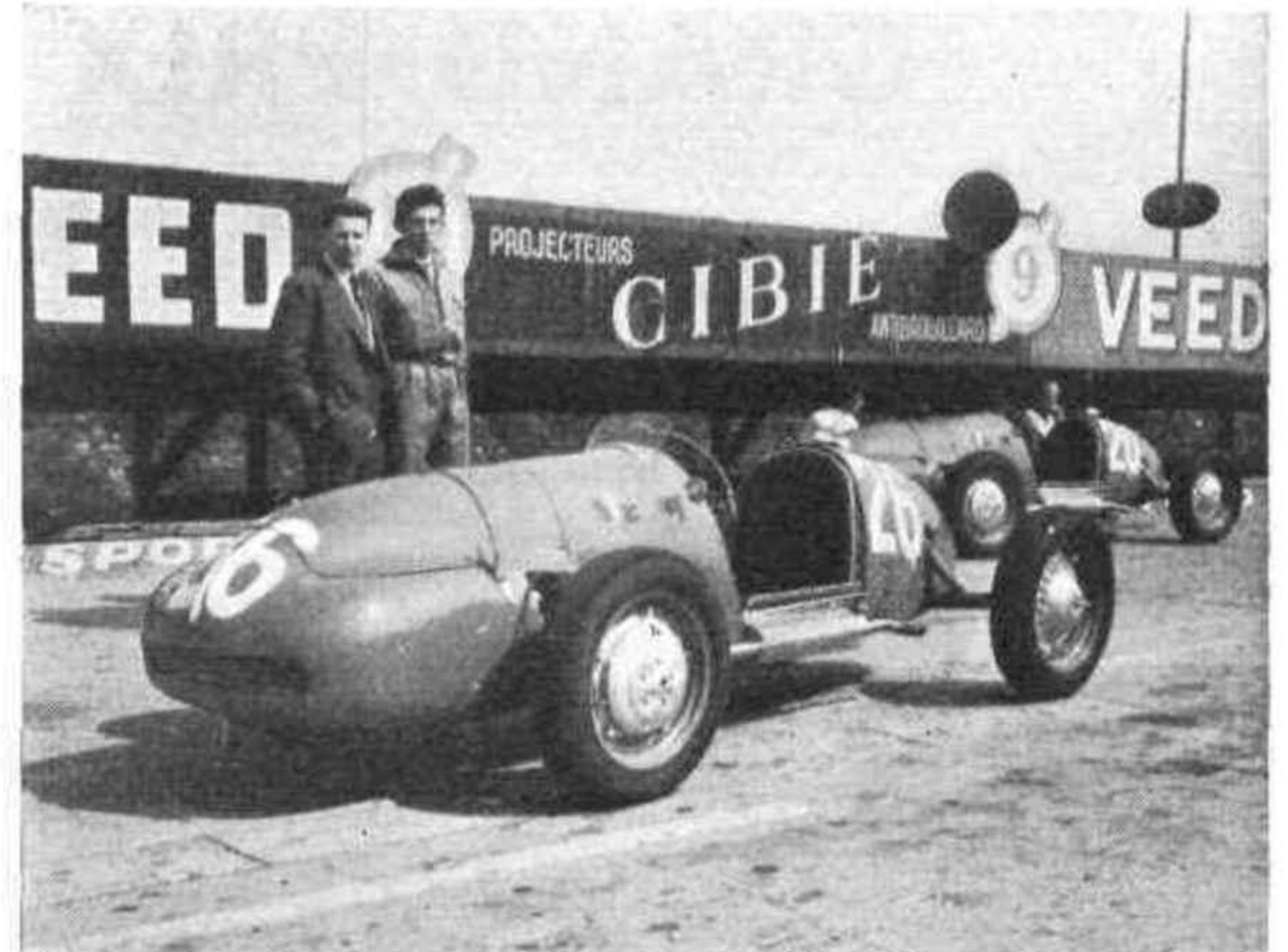
MONOMILL. —One of the strange vehicles constructed by René Bonnet to provide a "racing school" for young French drivers. The complete power unit is ahead of the front-axle line and the nose cowling is of a plastic material.
