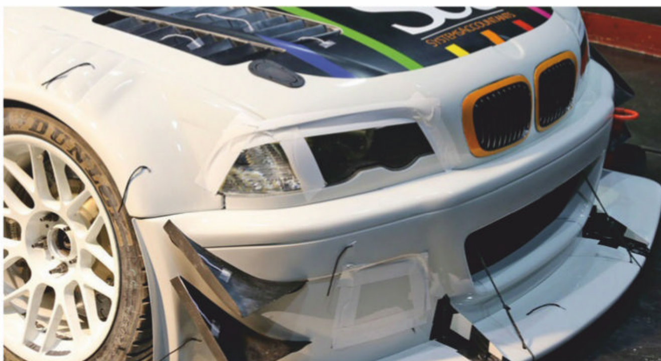
Using the race tape worked very well once again. Here the BMW's brake cooling ducts and its headlight gaps are covered
