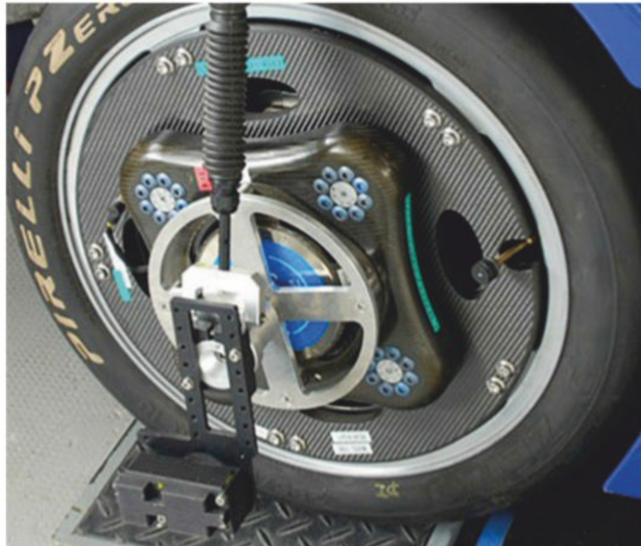
Slip angle sensor; the wheel force transducer measures all tyre forces and moments
