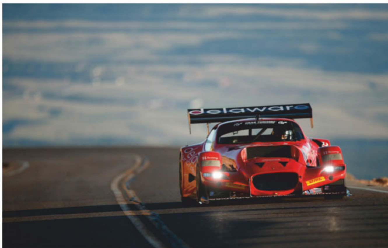
The Gillet Vertigo, a full-natural fibre bodied racecar, competed at Pikes Peak last year, getting to the top in under 11 minutes
