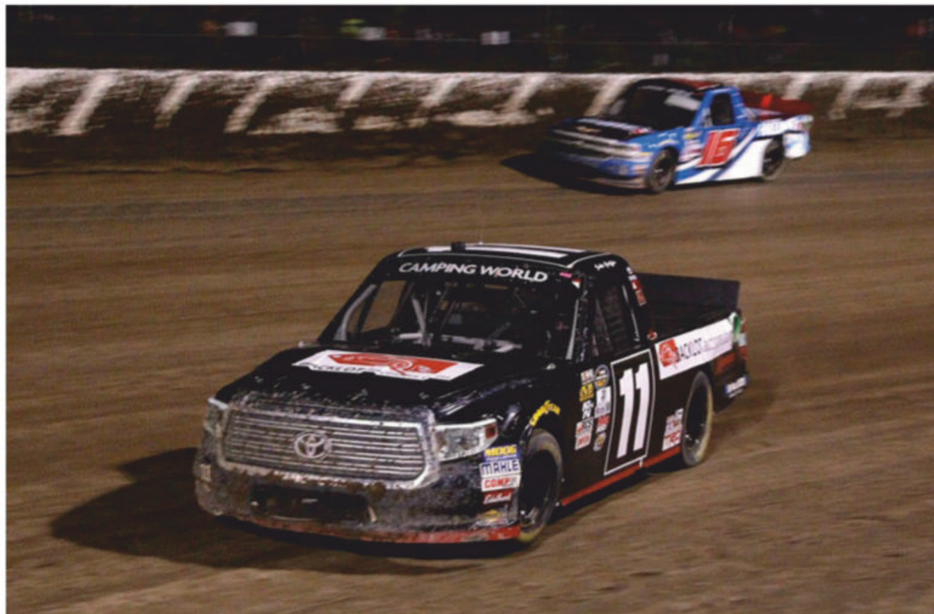
On dirt tracks a bias to the rear brakes is often useful on turn-in to help rotate the car. There can also be plenty of lateral bias
