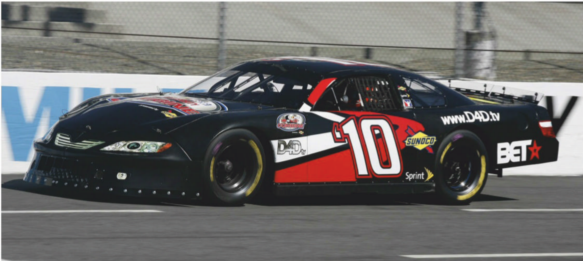
A NASCAR Late Model in action. When fuel is used up throughout a race the weight distribution will change and the brake bias will need to be adjusted to account for this
