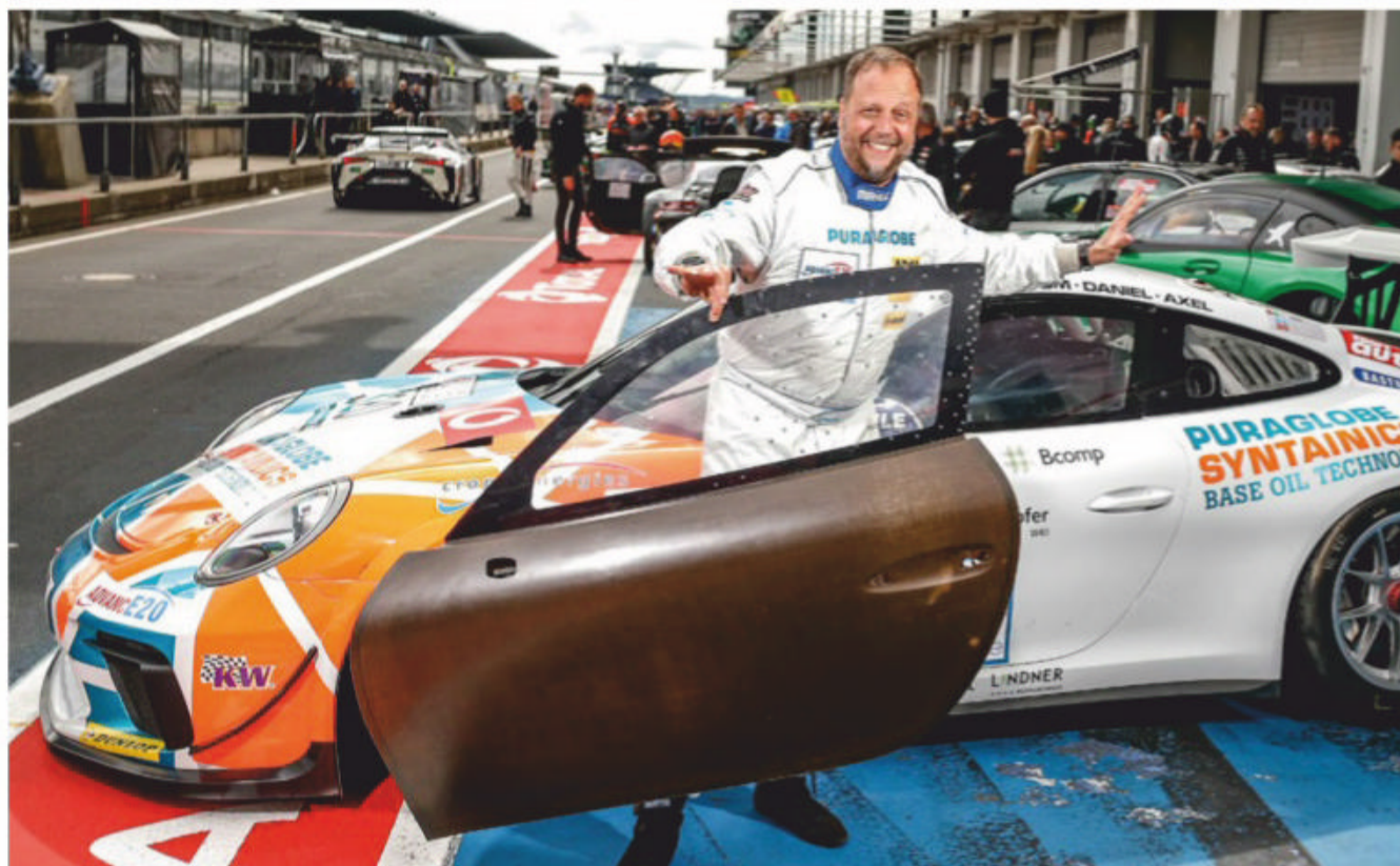
A natural fibre composite door panel for a VLN Porsche; these materials are best suited to semi-structural areas on the car
