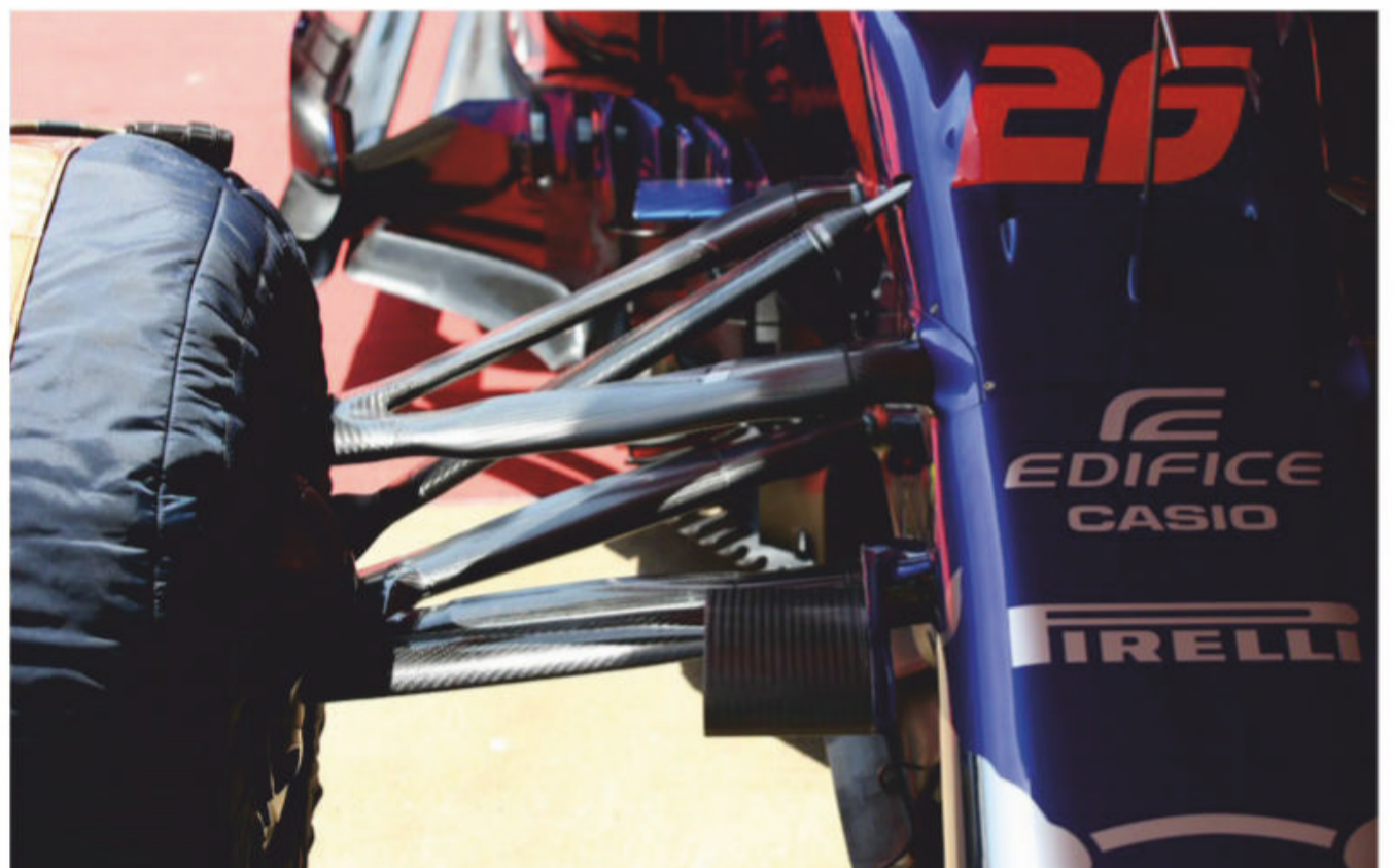
New front wing and end plate regulations have meant that Toro Rosso has had to rethink its wishbone design for this year
