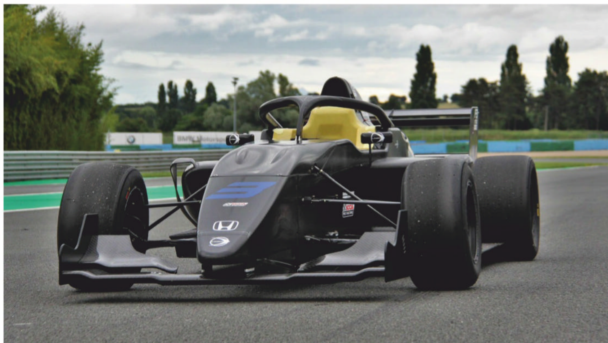
The Ligier JS F3R. Halos are mandatory while the design of the nose is tightly controlled for safety reasons. This means that all F3R racecars will look very similar from the front
