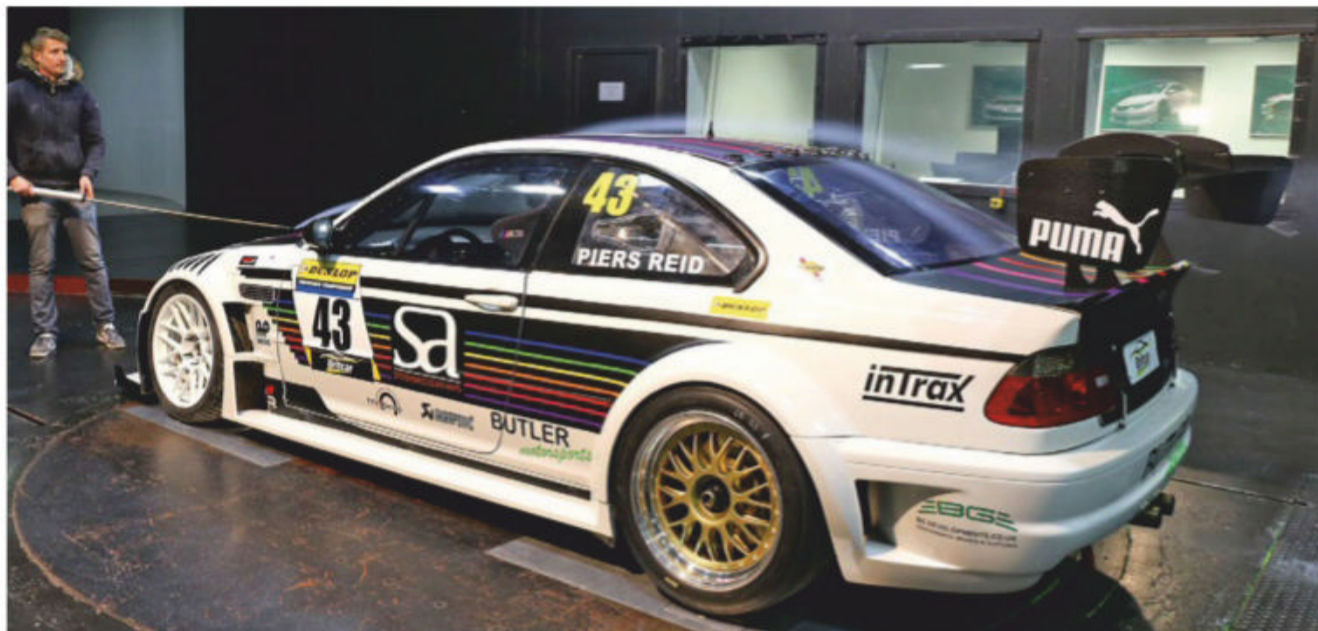
The M3's owner using the smoke plume. The objective of the session was to reduce the drag and find a better aero balance
