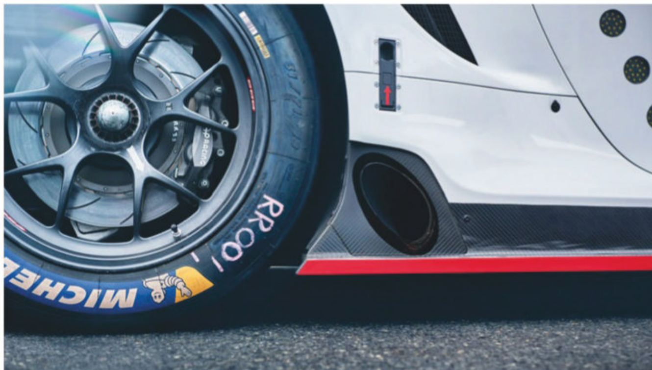
Side exhausts are a stand-out feature. Porsche says these help boost engine torque while also bringing packaging benefits
