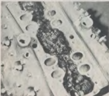
Sludge is caused by Water in the Oil
