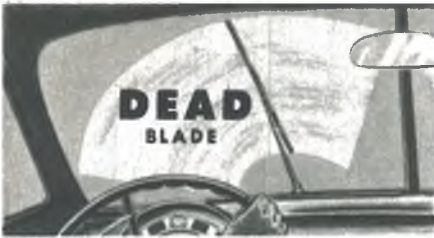
THIS DEAD WIPER BLADE still may look okay but it streaks glass dangerously.
