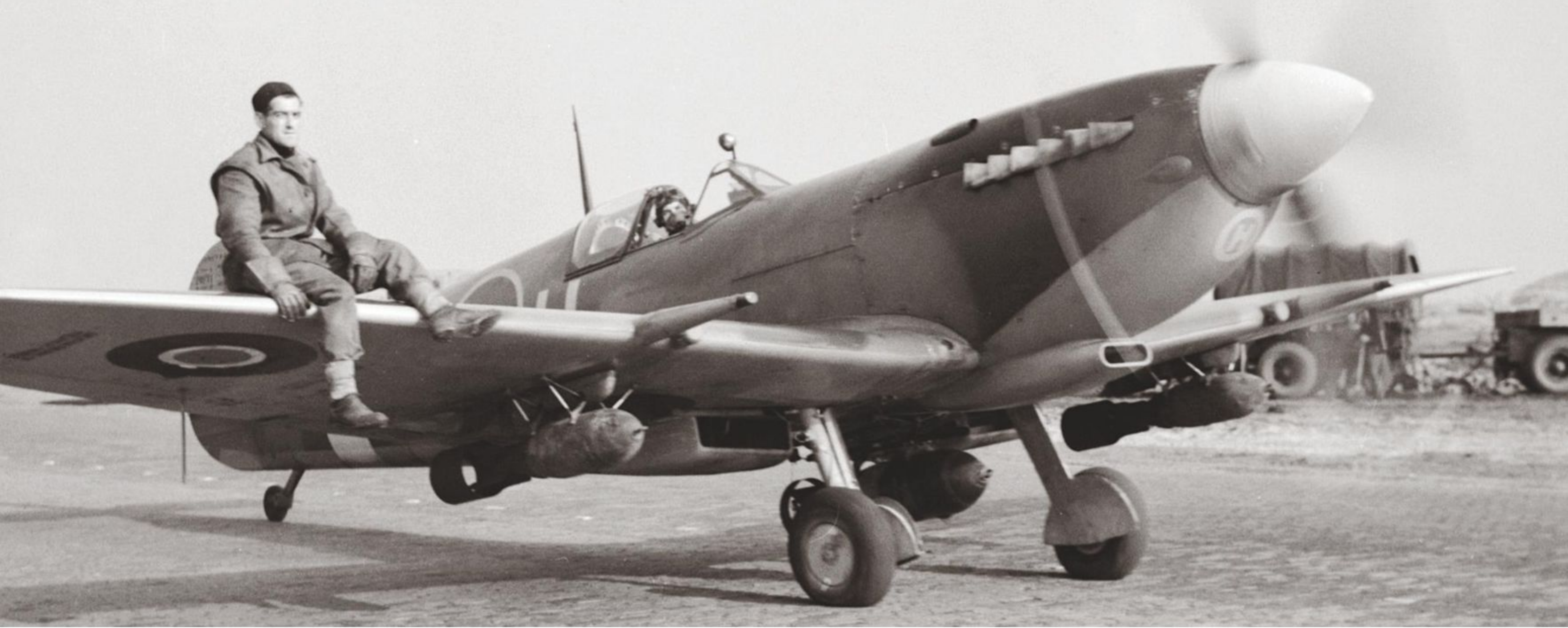
A wing rider guides a No. 412 Squadron Mk IX out with a full load: 1,000 pounds of bombs (one 500- and two 250-pound bombs). The wing-mounted 250-pound bombs were of questionable tactical value due to their low explosive weight. (Photo courtesy of Donald Nijboer)
