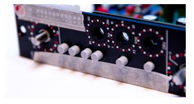
Now we will cut the LEDs legs. Make sure you have the right leg for + and - ( Long leg is + and short leg is -). I usually don't cut them straigt and keep two different size legs, so you still know which leg is + and which is -.
