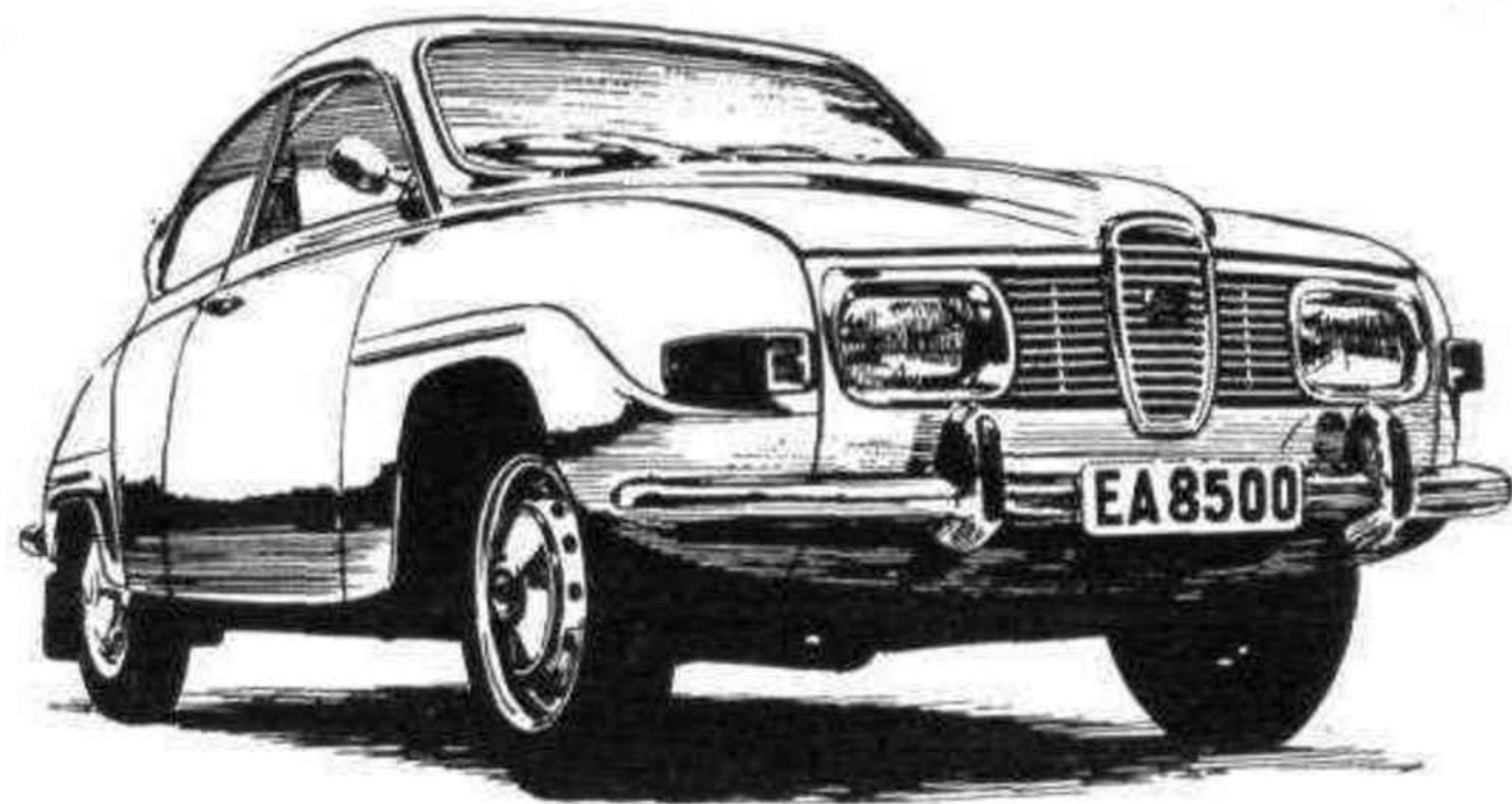
The lean low-drag aerodynamics of the Saab 96 have remained unchanged for 21 years, the body shape having been used for the original Saab 92s.
