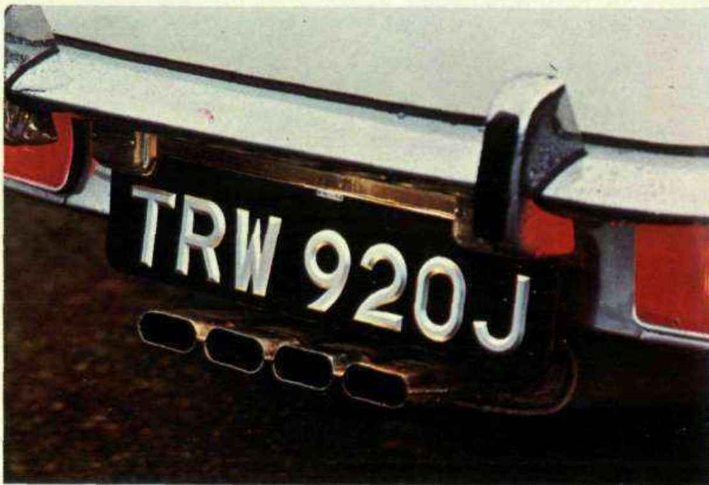
The four megaphone-type exhaust tail-pipes which whisper the music of the Jaguar V12.
