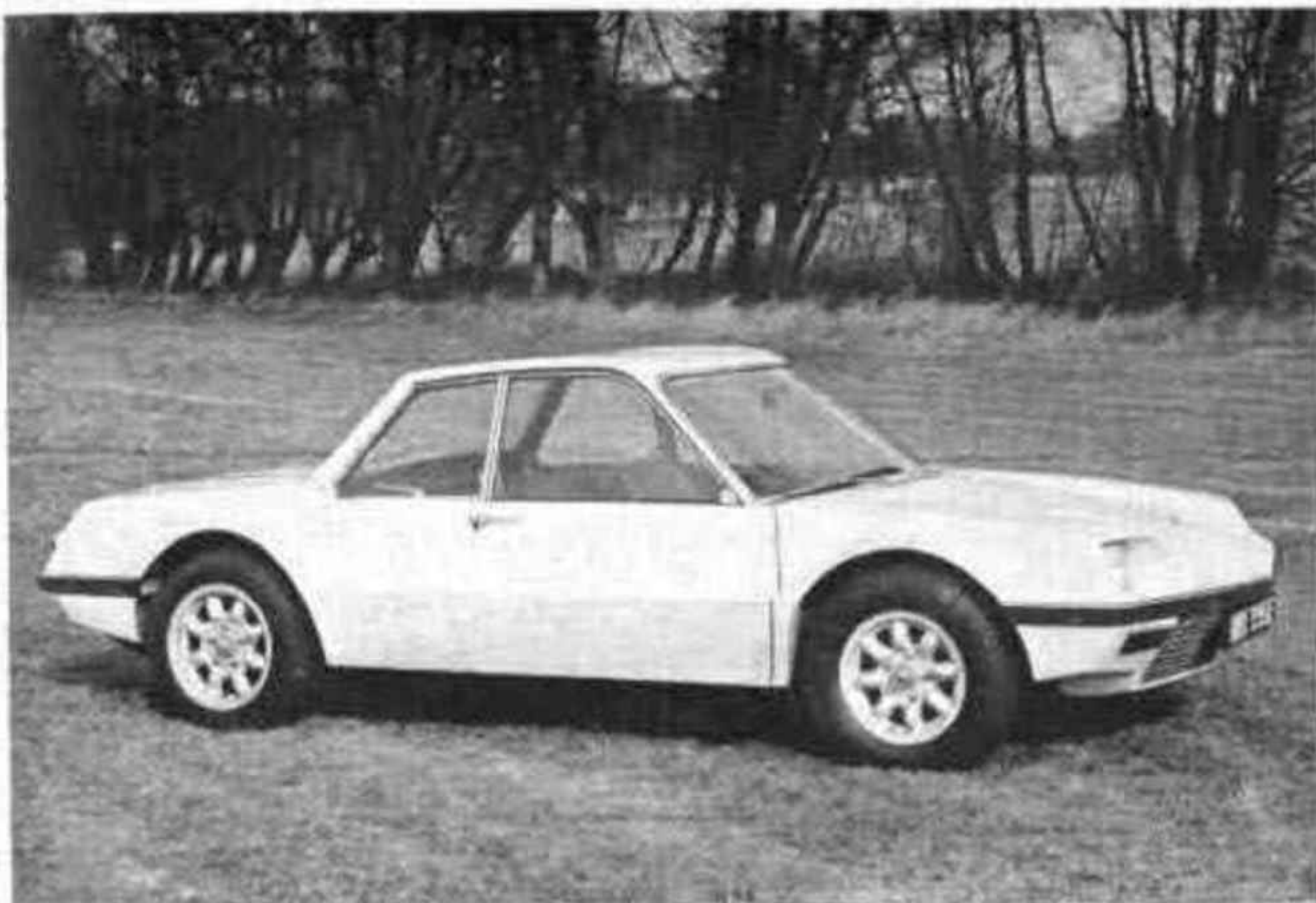
WHAT MIGHT HAVE BEEN. —The Rover BS coupé, with its V8 engine mounted over the rear axle and gearbox ahead of it, giving ideal weight distribution and a spacious cockpit.
