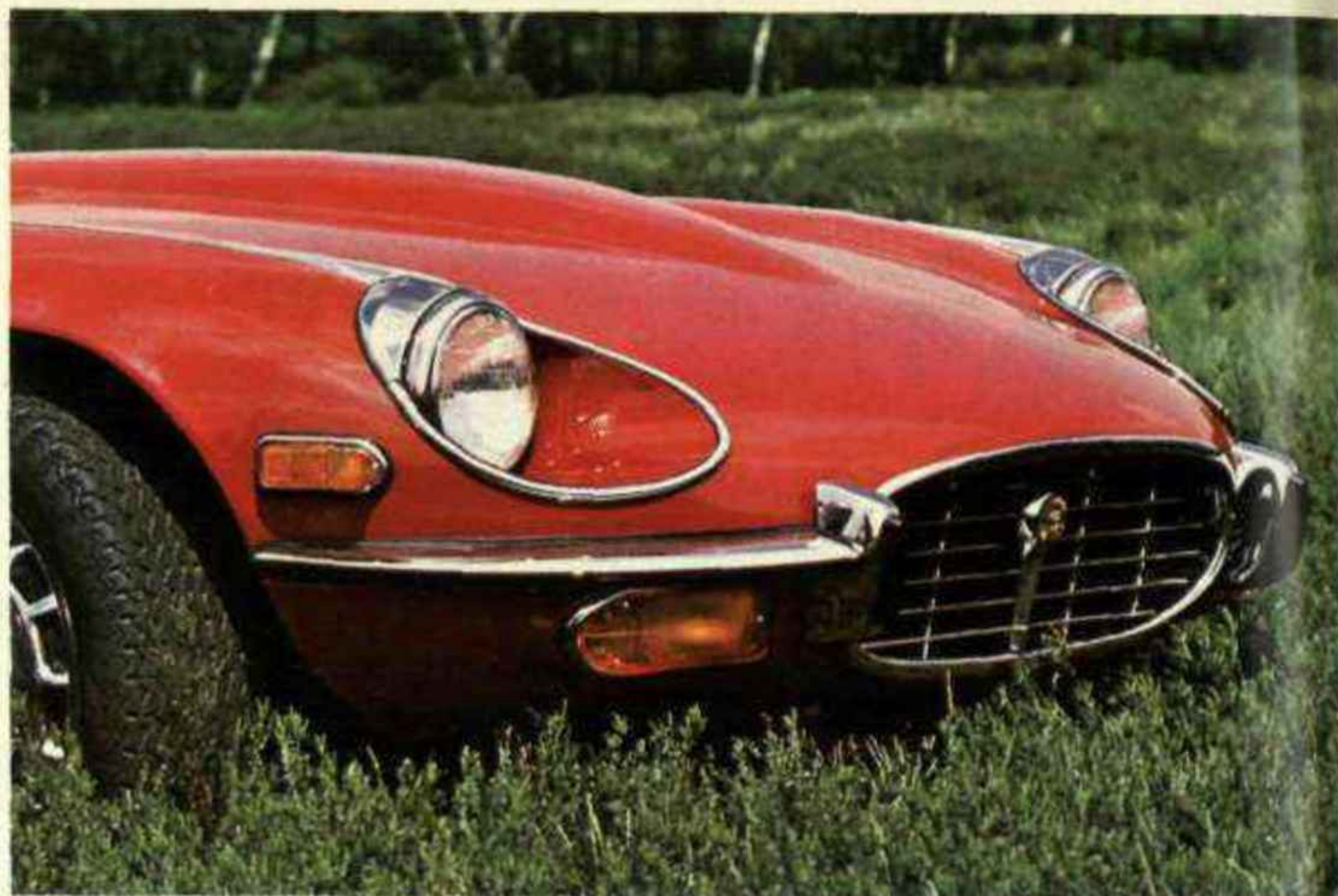
The decorative bird-cage grille stuck up the nose of the Series III 'E'-type Jaguar.
