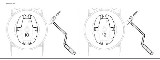
Plug in the crank and turn until it engages
