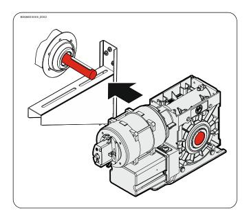
► Tighten all connection elements (M12) to 75 Nm. Install all other connection elements according to the specifications of the door manufacturer.
