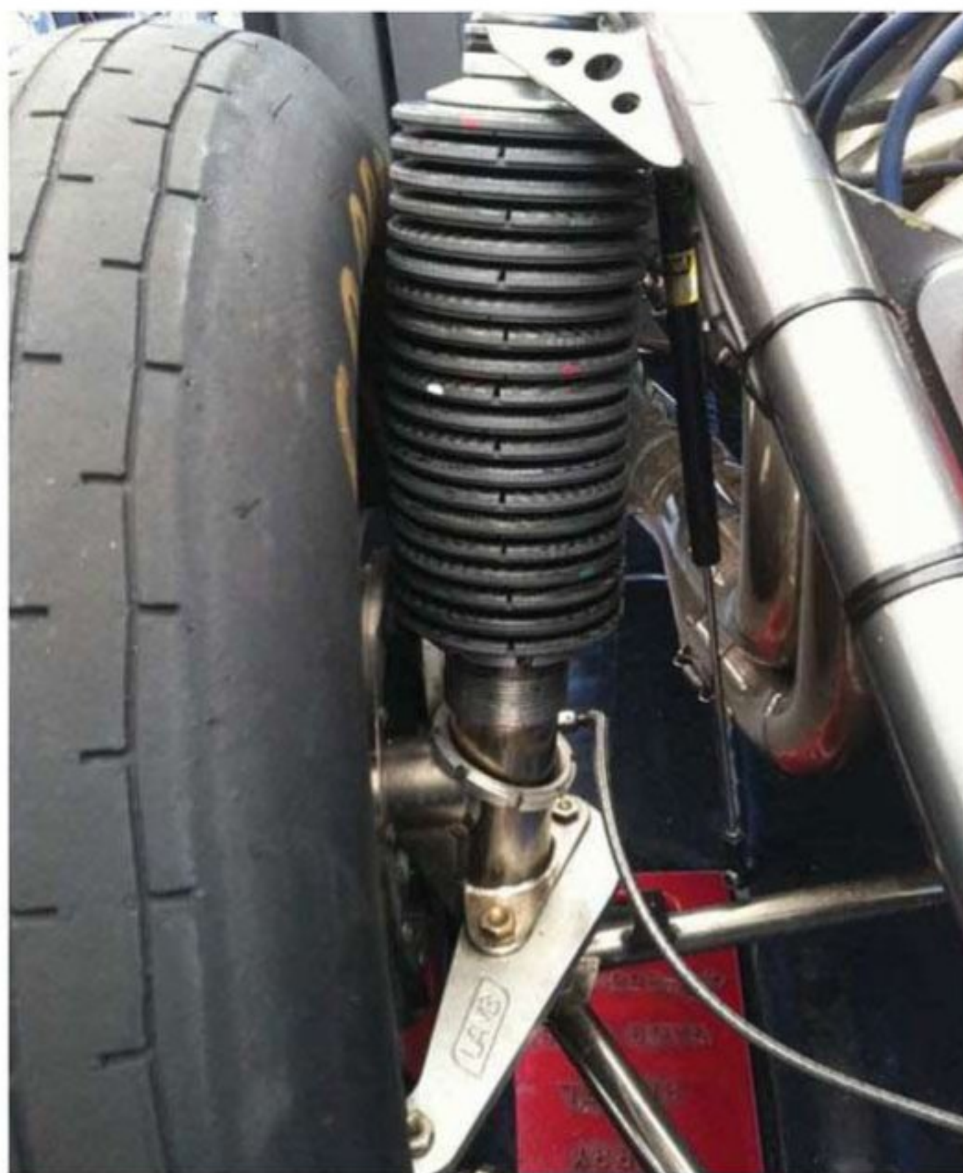
The benefits of carbon springs are multiple, but a less obvious one is reduced side loading on the damper shaft, improving damper efficiency
