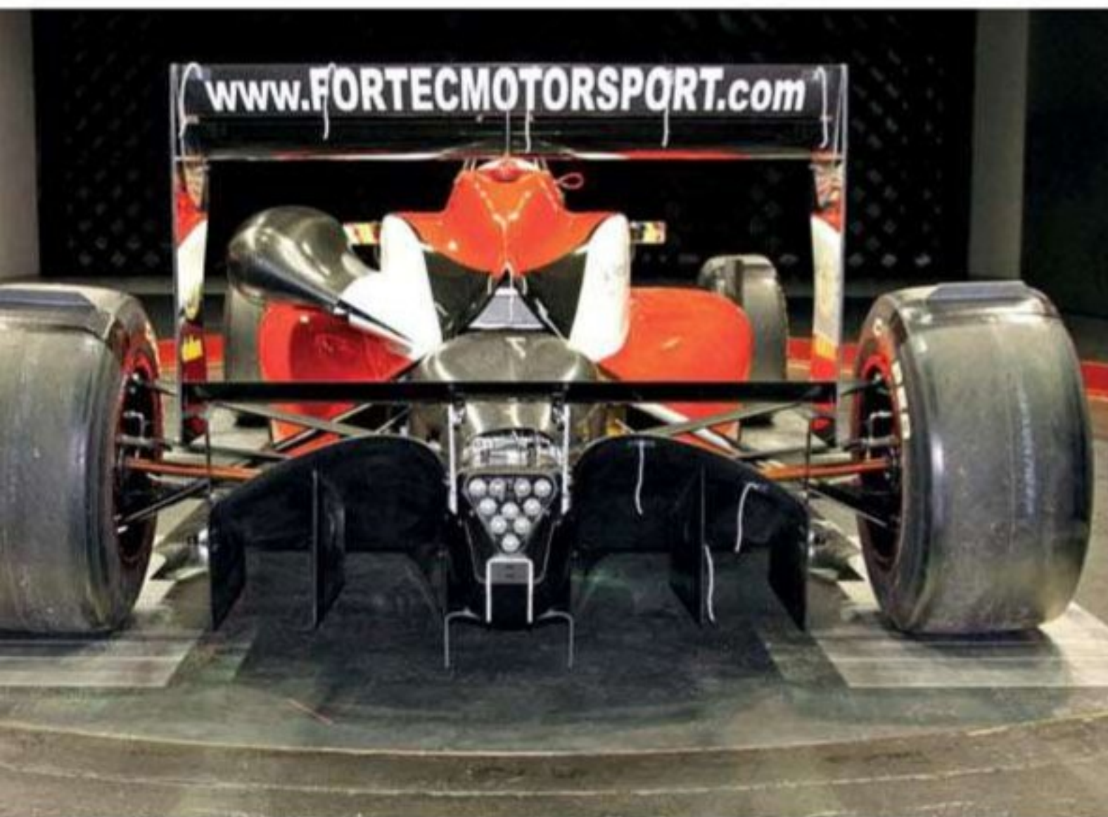
The 2012 Dallara F312 rear diffuser looks similar but the lower, centre section is narrower, the rear light has been more tidily located and it is missing one or two details visible on the earlier car's diffuser
