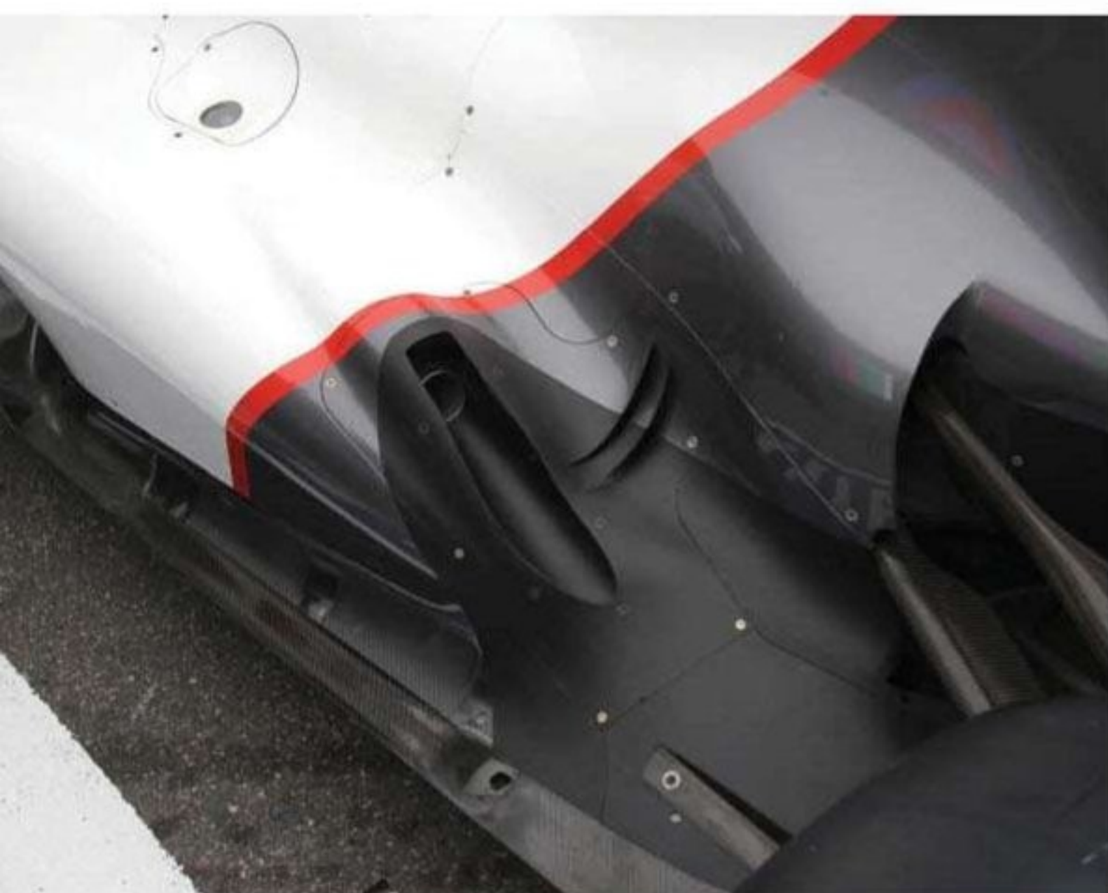
Innovative exhaust design essentially acts like a blown diffuser, and has since been copied by a number of other teams on the grid
