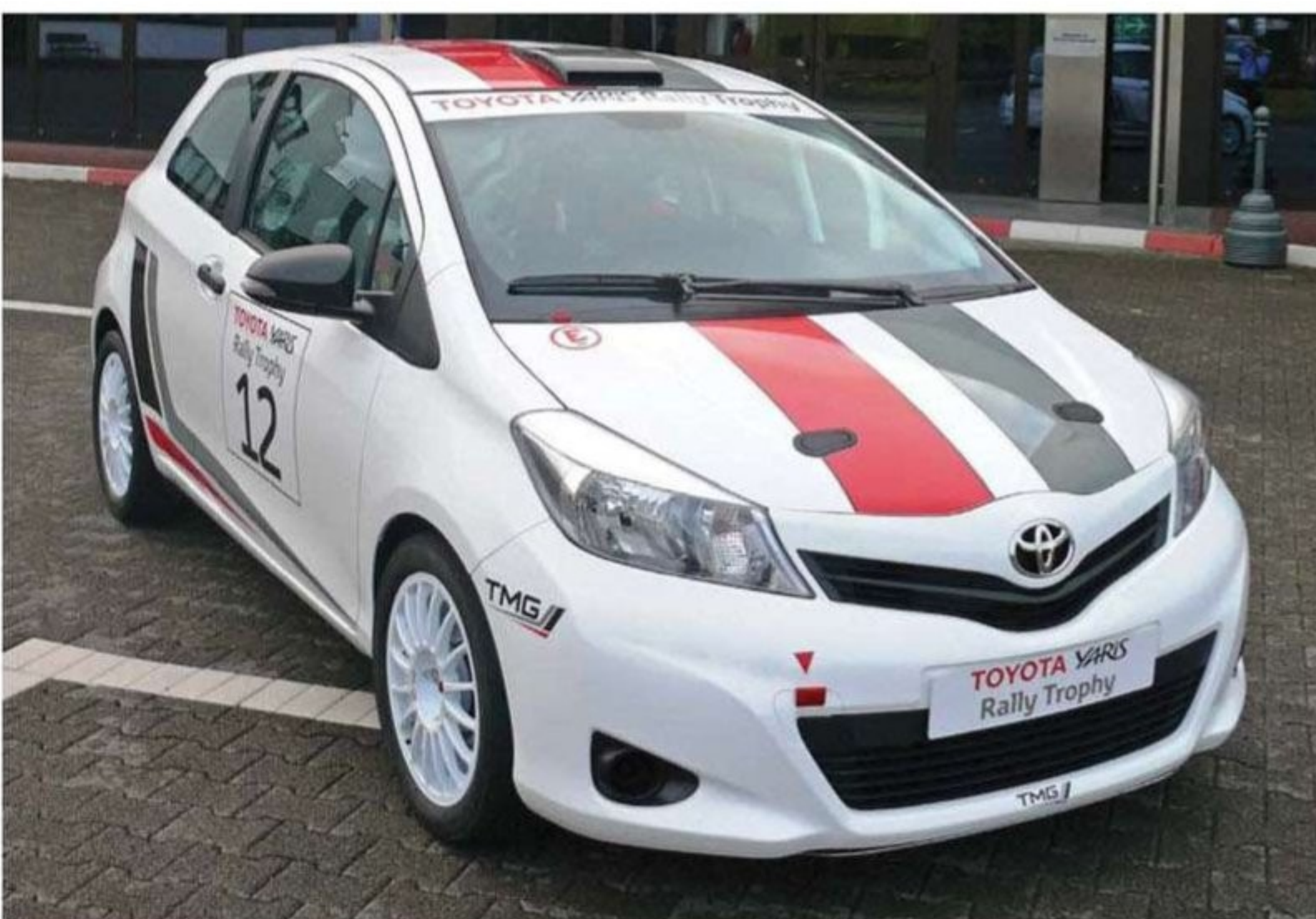
The Toyota Yaris uses the same engine and gearbox as the road car, although the final gear is slightly shorter
