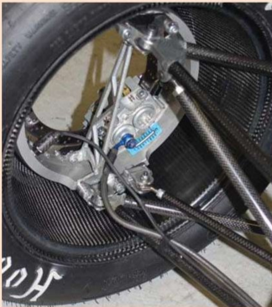
A huge 400g per hub weight saving made the centreless wheel concept worth pursuing. The team also claim a greatly decreased load path distribution through to the front wishbones
