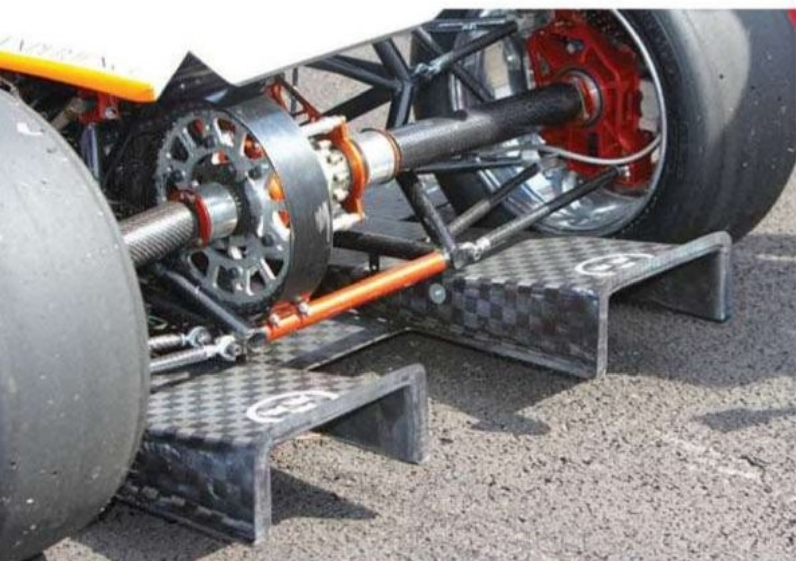
Karlstad University entry appeared with no wings and just an underfloor diffuser, which proved to be the quickest overall solution in the dynamic events, as shown by a similar treatment on the Munich and Stuttgart entries
