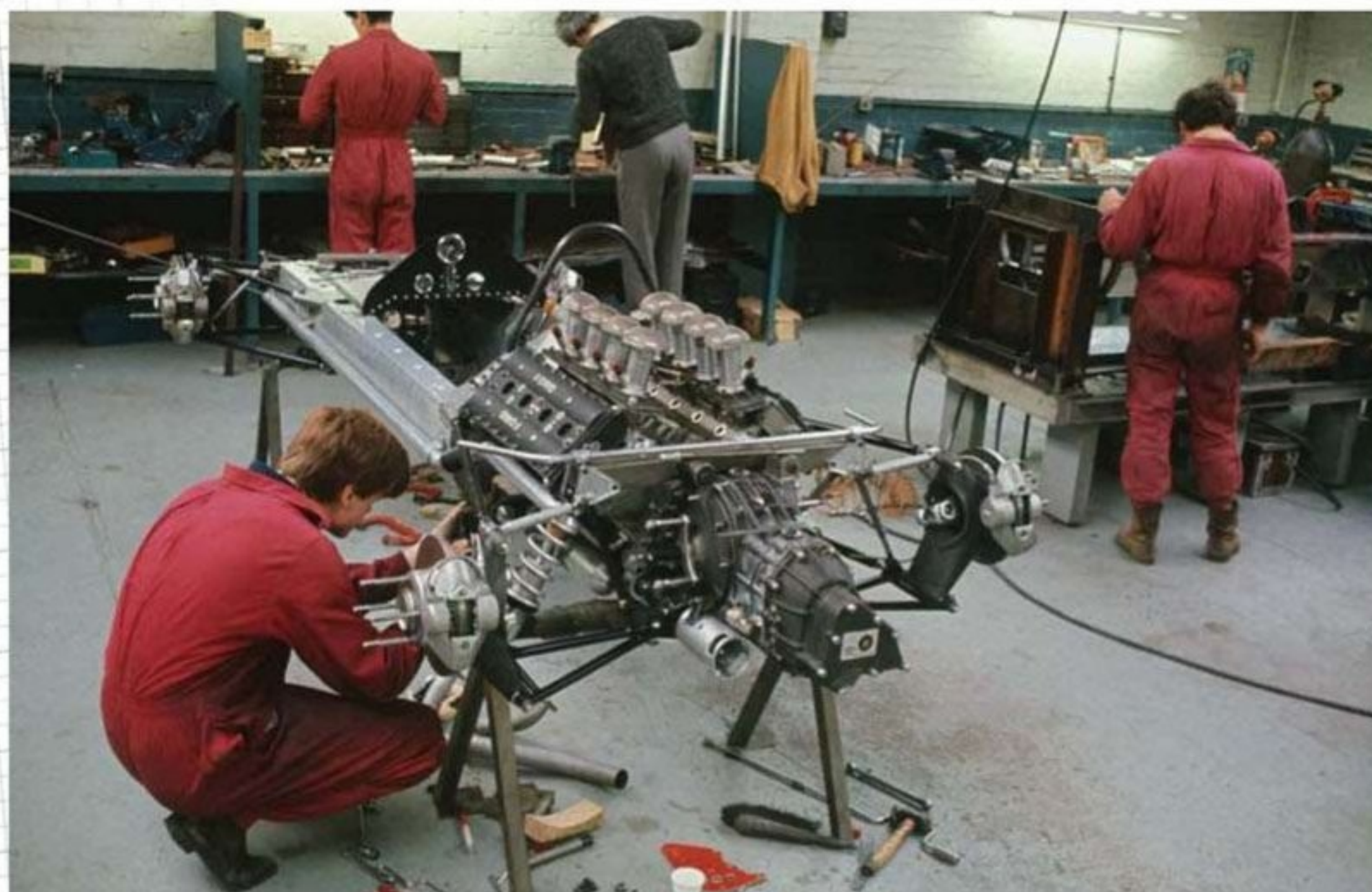
A Ford DFV-powered McLaren M7A under construction at the Woking facility in 1968
