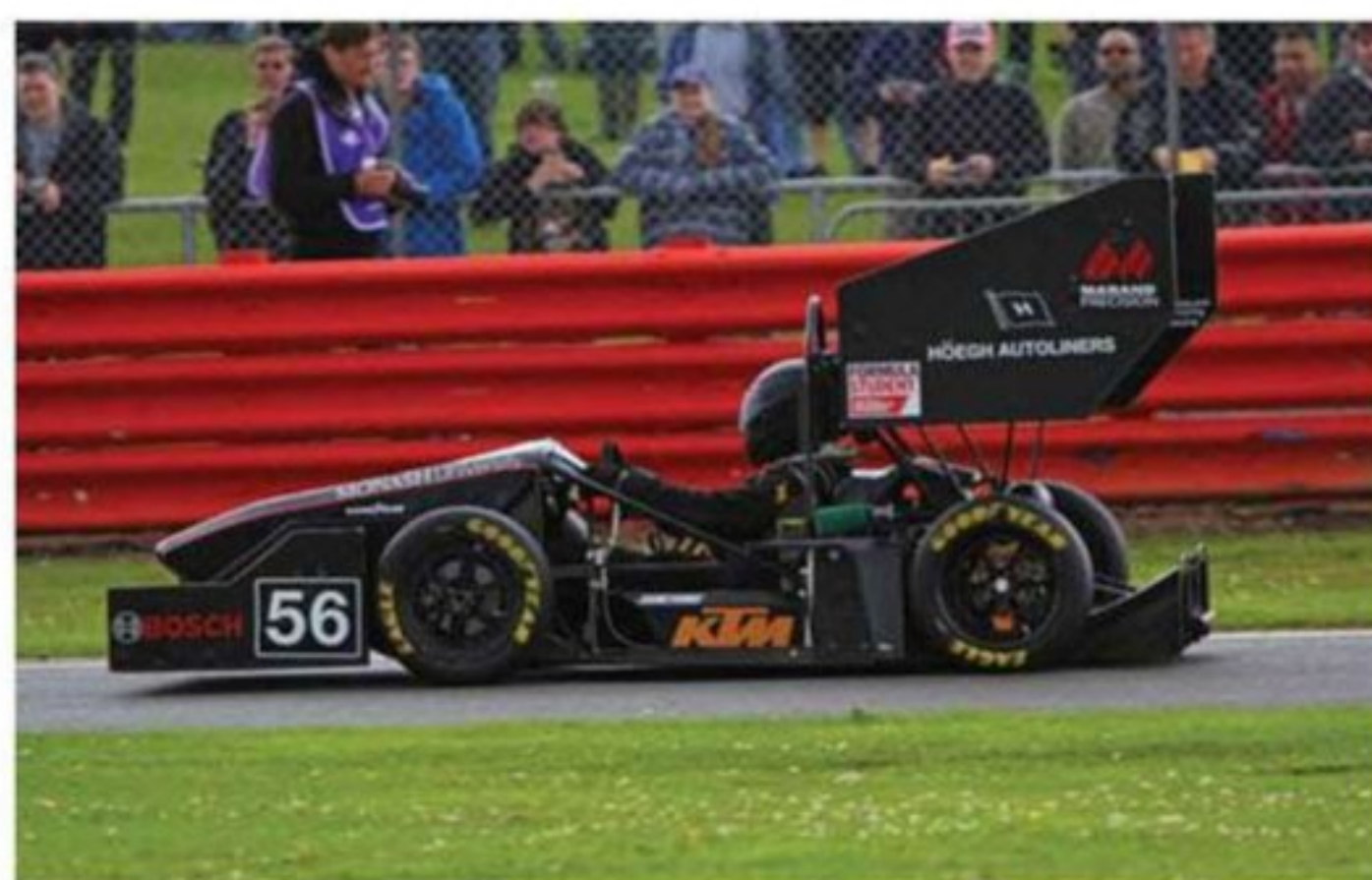
The Monash car had adjustable wing flaps to alter the attendant drag penalty
