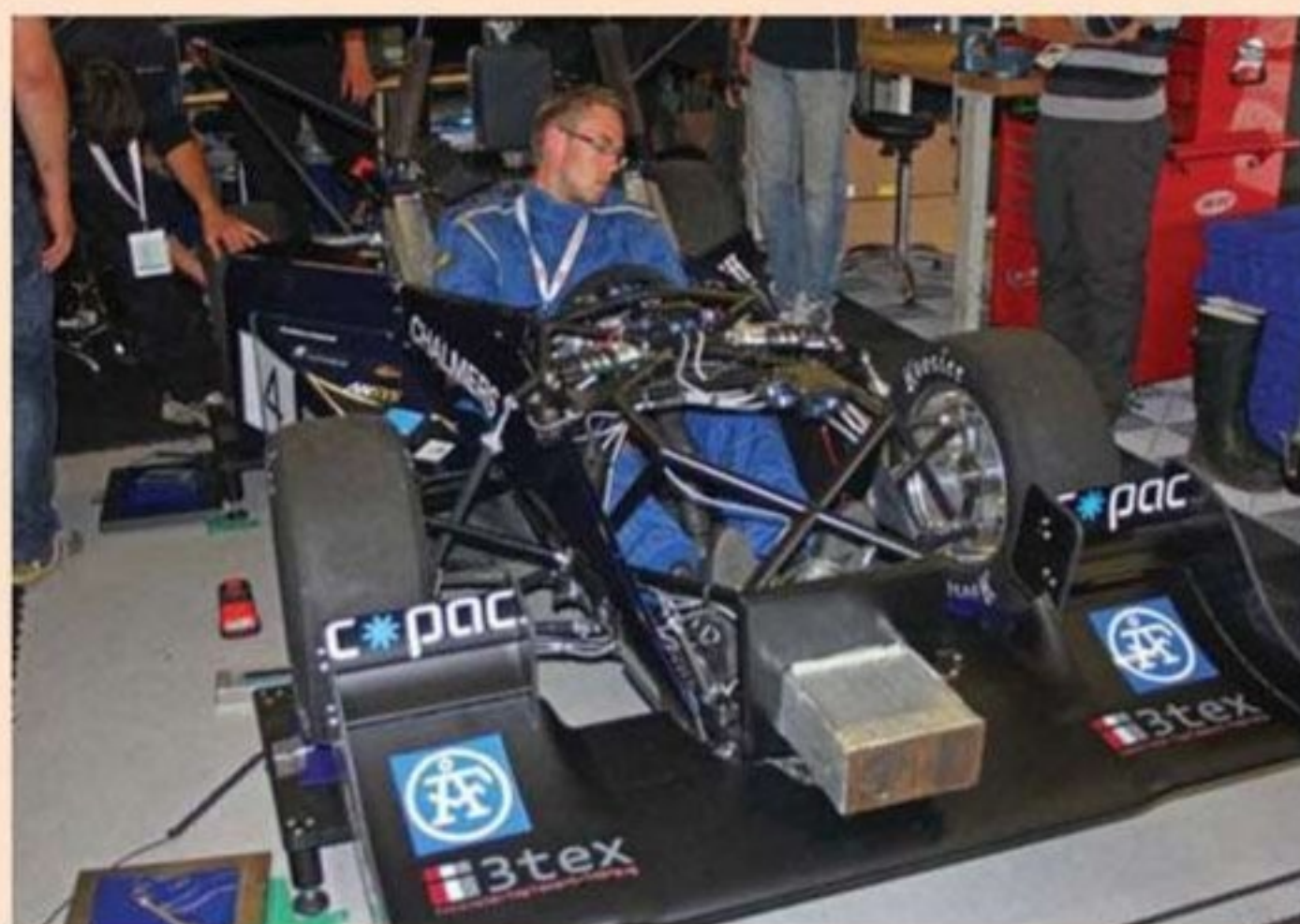
Weight has gone up, but so has chassis stiffness, from 800 to 3800Nm/degree
