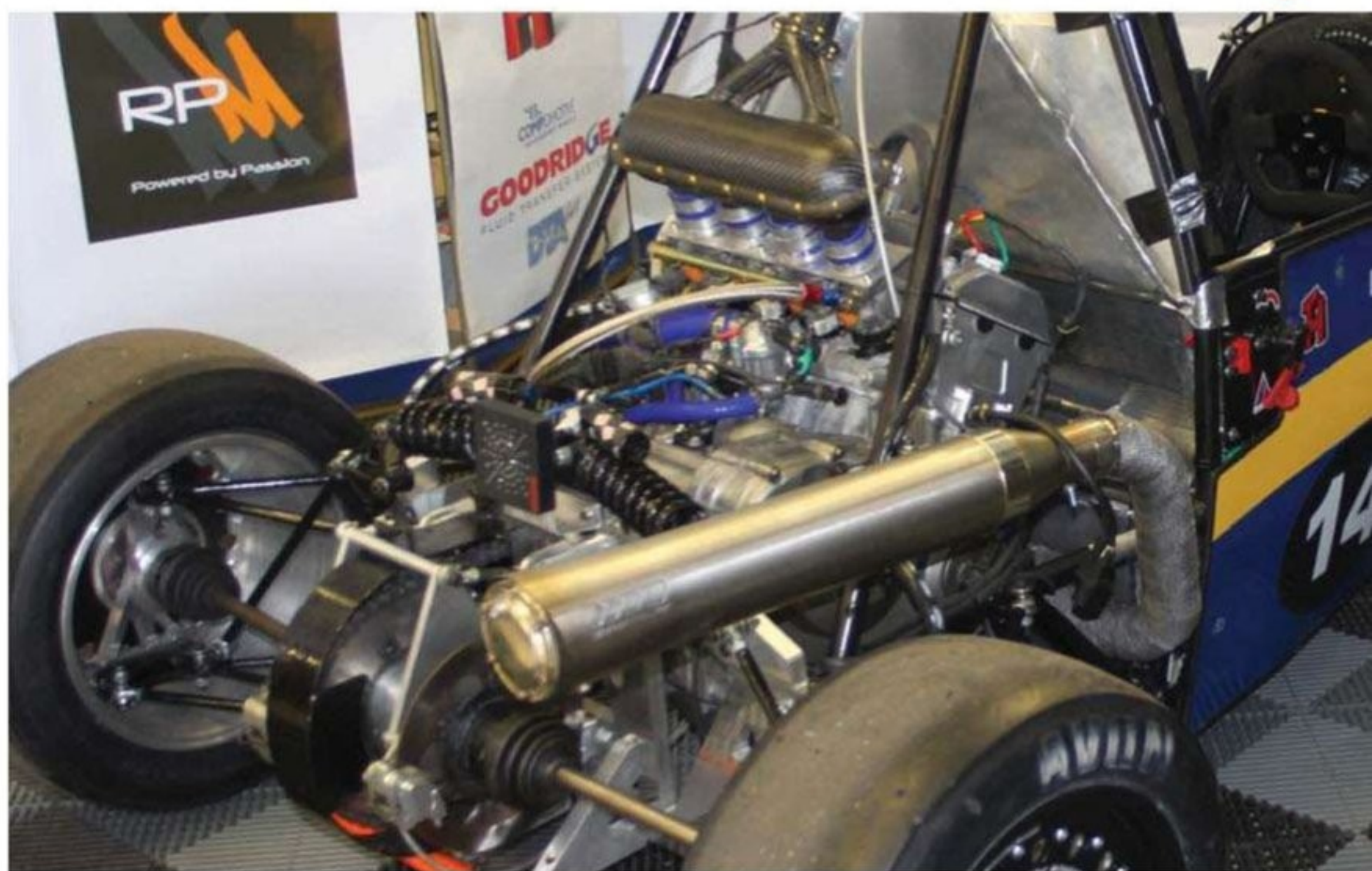
Herriot Watt Racing stuck with the more traditional Formula Student layout, utilising a 2006 Honda CBR four cylinder
