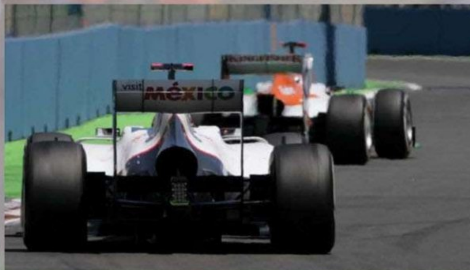
Hot track set up has a large cooling aperture at the rear (above), while that aperture is made significantly smaller when running at cold tracks
