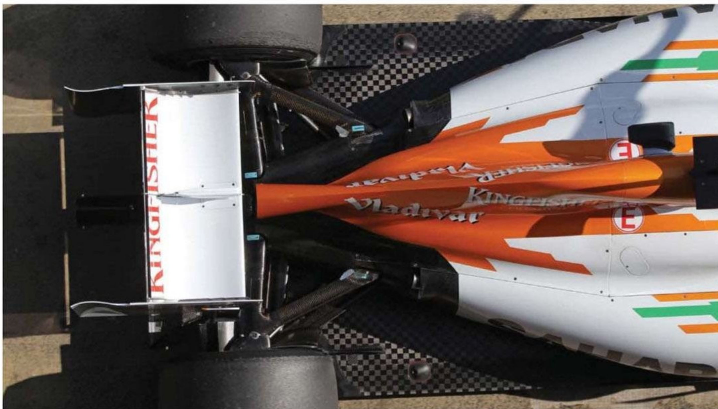
Exhaust detail was deliberately conservative on the launch-spec car, the team waiting until the FIA clarified what was legal before bringing out...
