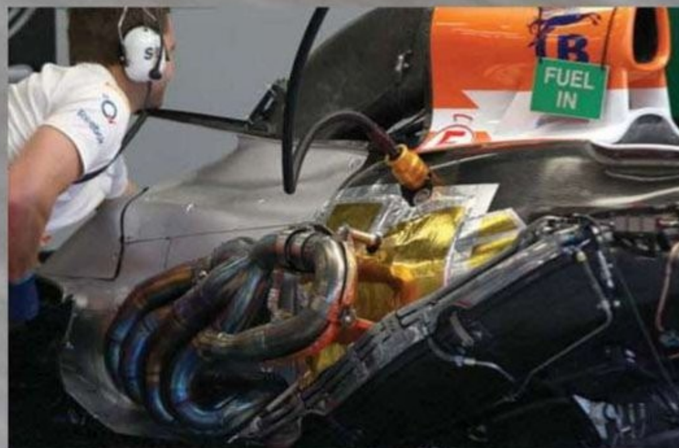
Sidepod, exhaust and engine bay layout shows how the aerodynamic concept carries through inside the vehicle as well as outside
