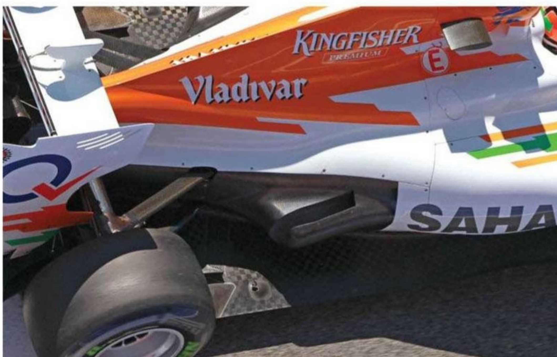
...this 'blown diffuser' version at Barcelona. It works, but has caused some balance problems for the drivers
