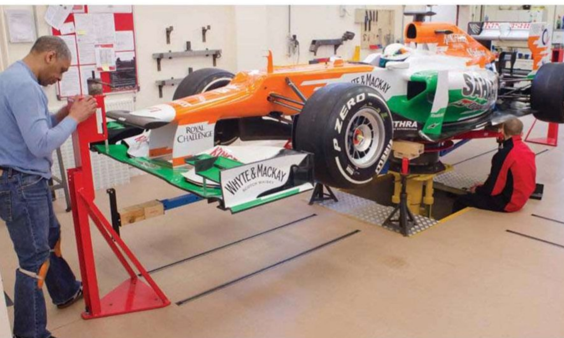
The Force India VJM05 on the Cranfield moment of inertia rig, which the team are using to test alignment in pitch, roll and yaw, as well as to measure c of g height and numerous other factors being used to develop the team's current F1 chassis
