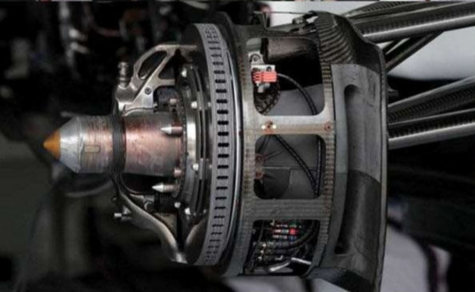
Top: central 'vent' is not a vent at all, but smooths airflow around the nose. Middle: packaging in the sidepods is a 'nightmare', and airflow through the radiators is controlled by blocking the system (see right), depending on track temperature. Bottom: continual development work goes into the cooling ducts on the C31's brakes, optimising them for different tracks
