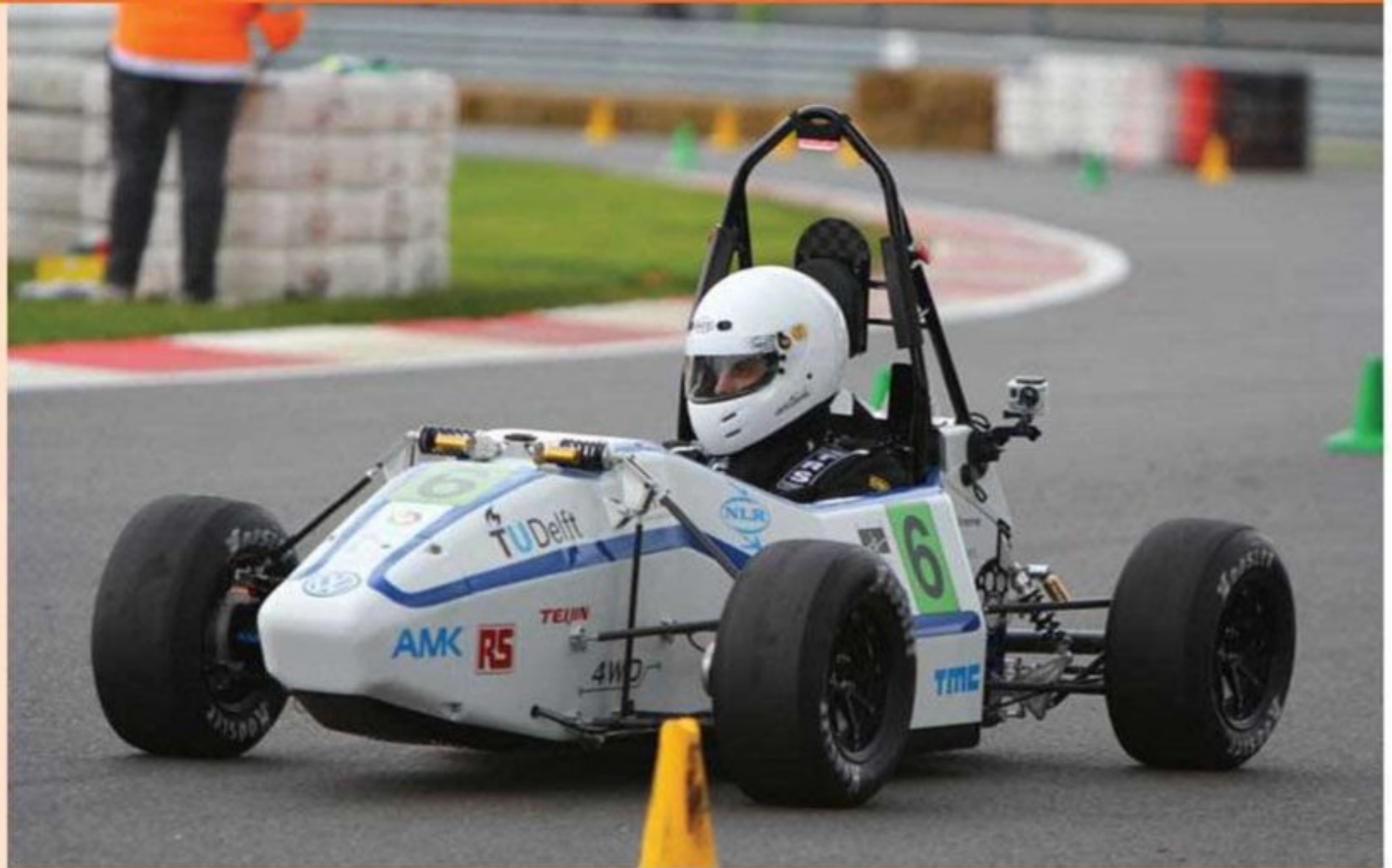
The lack of an aero package did not seem to hamper TU Delft's all-electric car, which also featured regenerative braking
