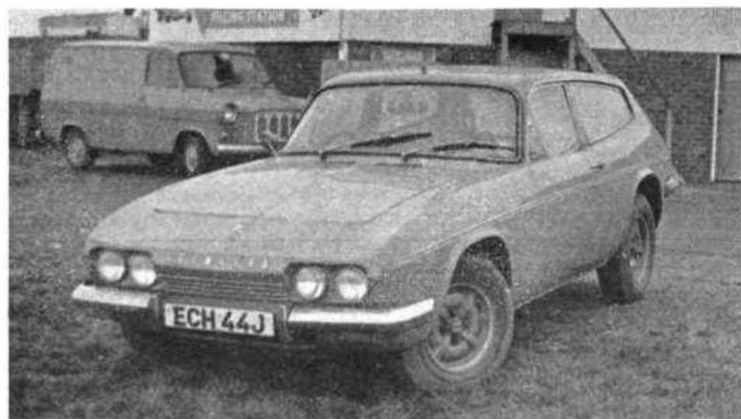
MUCH OF the car's life is spent travelling to racing circuits. Here the Scimitar GTE rests in the Mallory Park paddock. The trim strips along the side have tended to spring off but are not included on the 1972 model. The wheels have also been re-styled.
