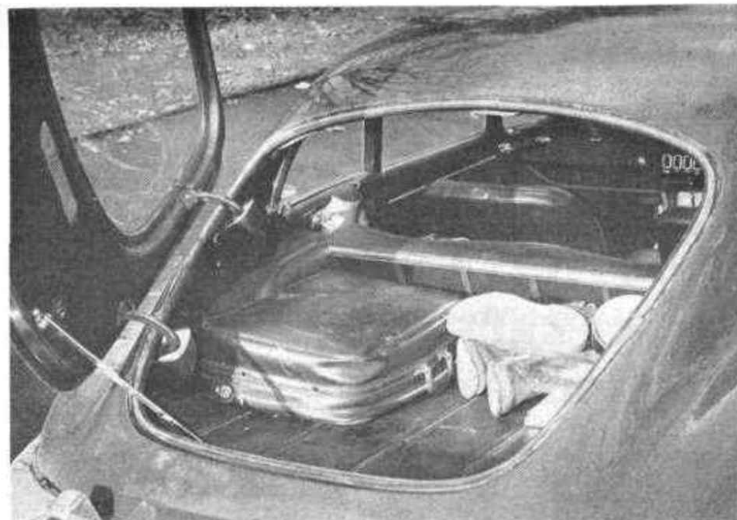
LUGGAGE SPACE on the V12 E-type 2+2 is on a platform below the hinge-up back window, the release for which is inside the car. With only two people in the 2+2 the rear seat back-rest can be slid forward to give increased storage space.
