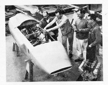
Since 1927 no one has had any success in the India-napolis "500" with a car powered with a production U.S. engine. The Mickey Thompson organization have accepted the challenge. The men, left to right, with the lightweight, rearengined, Buick V8powered machine are Jack "Willy" Sutton, Glenn "Red" Rose, John Crosthwaite, and Don Borth, The Don Borth. 330 b.h.p. engine is below.
