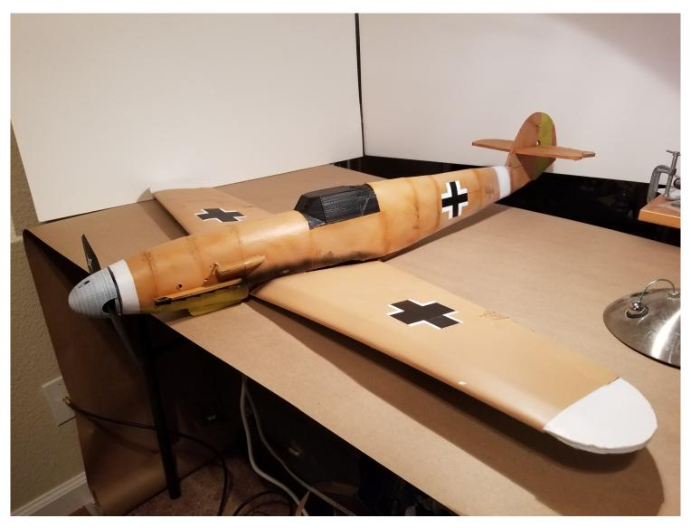
I suggest that you print this in black and white and skip the last pages that have images instead of stencils to save your printer ink. Note that the hole for the motor mount are measured for a flight test C-Pack motor, the GT2215/09. Also, be aware that your skin stencils may vary due to build imperfections so always cut bigger than your need and trim down after gluing.
