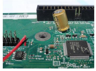
While heating up one pad at a time, apply pressure to the cap so it breaks free. You may need to do this a couple of times rotating between the two pads until the ClockCap is completely removed.
