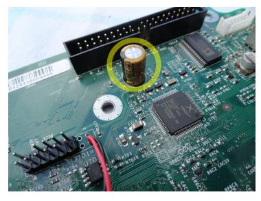
Version 1.6 console ClockCaps are located right next to the IDE connector and clearly stands out. These ClockCaps are "Nichicon" which are one of the best capacitors you can get. I have ever seen these ClockCaps leak and shouldn't require removal. From memory version 1.6 consoles wont boot or work correctly without a ClockCap.
