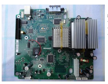
Reinstalling the heat sinks is much easier than removing them. If you've made it this far the final step should be very straight forward.
