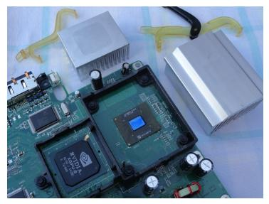
Again I had to apply heat to remove the old thermal compound, it was more of an adhesive. Use an old bank card or something plastic to scrap off the compound carefully. Next with a rag and isopropyl alcohol wipe off as much as you can before maybe going over it one last time with cotton tips
