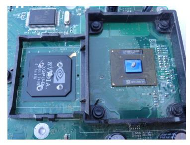
With everything cleaned up its time to apply some new thermal paste to the CPU and GPU. Just apply the one bead to the CPU and a few extra's for the GPU as shown in the image to the left. When the heat sinks are installed the thermal paste should spread out relatively even.
