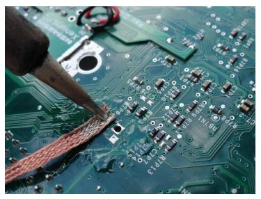
With the ClockCap removed use a solder sucker to remove the majority of the solder then apply flux and clear out the remaining solder from the through holes with some wick.
