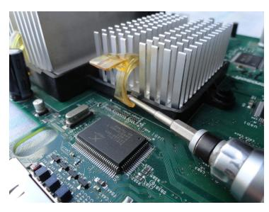
The plastic clips holding the heat sinks can be a little tricky to remove especially for the GPU. While applying pressure downwards on the thumb tab, you will need to use a flat head screw driver to assist in process as shown in the image to the left.
