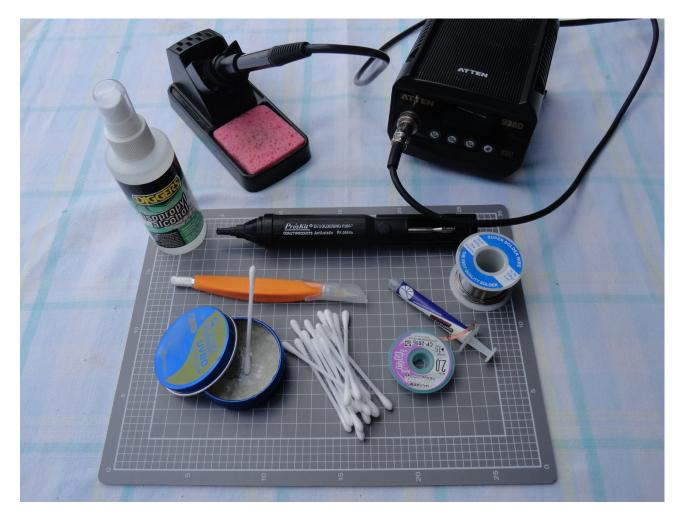
A good soldering iron with temperature control will be a huge benefit. My general rule of thumb is to use 340°C for general soldering, 360°C for desoldering and 400°C for anything that's grounded. I like to use a 1.2mm tip on my iron with 0.8mm solder with 60% lead, be sure to use Flux as it will greatly improve the quality of your work. I recommend desoldering wick and a solder sucker. Some isopropyl alcohol, cotton tips and a toothbrush will assist with any cleaning.
