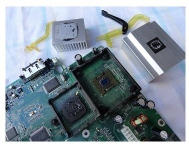
After removing the clips I still found it difficult to remove the heat sinks as they were pretty much glued in. In this case I probably didn't need to replace the thermal paste but I went ahead for the guide.
