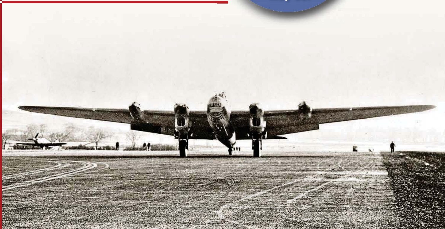
BELOW: The Pe-8's wingspan of 128ft 4in (39.13m) was greater than that of any contemporary operational British or American four-engine bomber, although the B-24 Liberator's slender Davis wing of 110ft (33.5m) came close. Note the Hurricane seen here in the background at Tealing, home to the RAF's No 56 Operational Training Unit. Philip Jarrett collection
