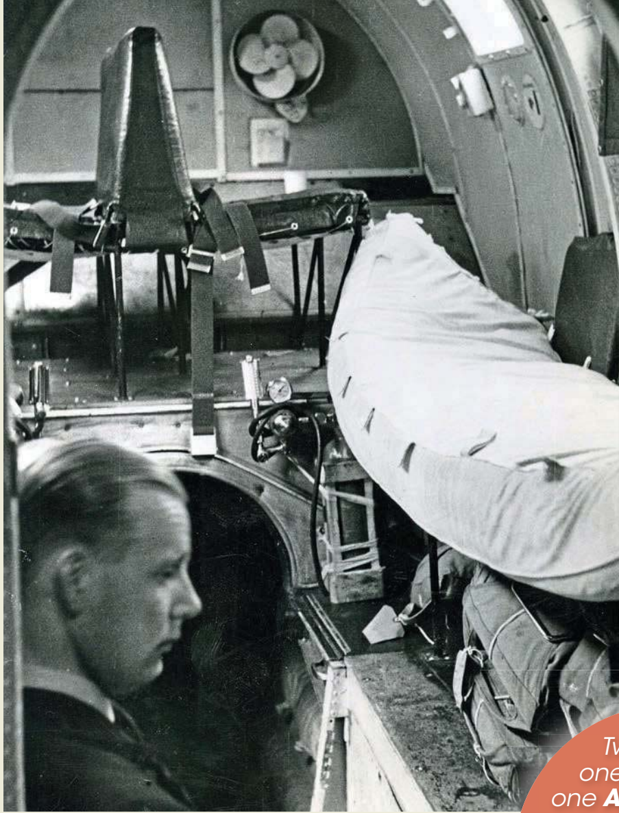
ABOVE: Typical accommodation looking aft in the cabin of a Ferry Service Liberator, with side seats in the rear of the cabin, bunks in the bomb bay and a shelf - known as the "Bridal Suite" - above the bomb-bay. TAH Archive
