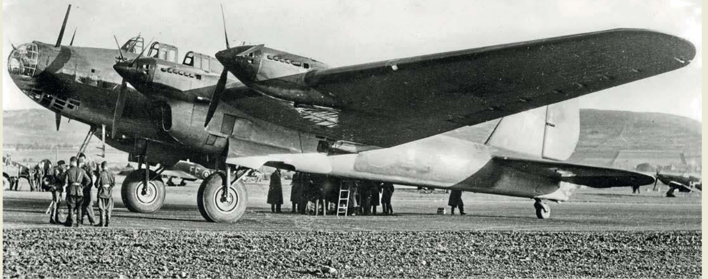
ABOVE: The mighty four-engined Pe-8 at Tealing on May 20, 1942. The Pe-8/TB-7 prototype made its first flight on December 27, 1936, the type becoming the only four-engined bomber built by the Russians during the Great Patriotic War. The Pe-8 that brought Molotov was a standard production example, fitted with four 1,340 h.p. Mikulin AM-35A V12 liquid-cooled engines. Philip Jarrett collection
