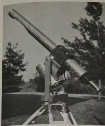
FIG. 84. Oscar Knab's mahogany and jeweled-aluminum Schiefspiegler (oblique reflector) on its altazimuth mounting is particularly valuable for lunar and planetary observing because of its excellent image quality. It is less well suited for viewing dim extended objects, such as galaxies and nebulae, because its focal ratio is high.
