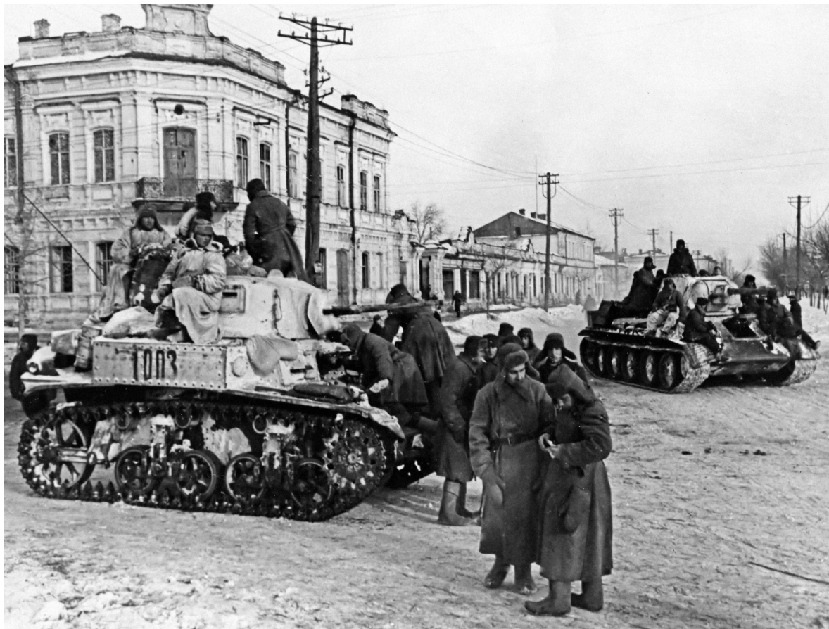
An M3L of the 23rd Guards Tank Brigade of the Western Front in Belgorod in February 1943 with a T-34 behind. This is from the fourth production series with the interim D58101 turret.
