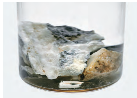
A large white portion on the stone does not lead to a substantial rise in total hardness.
