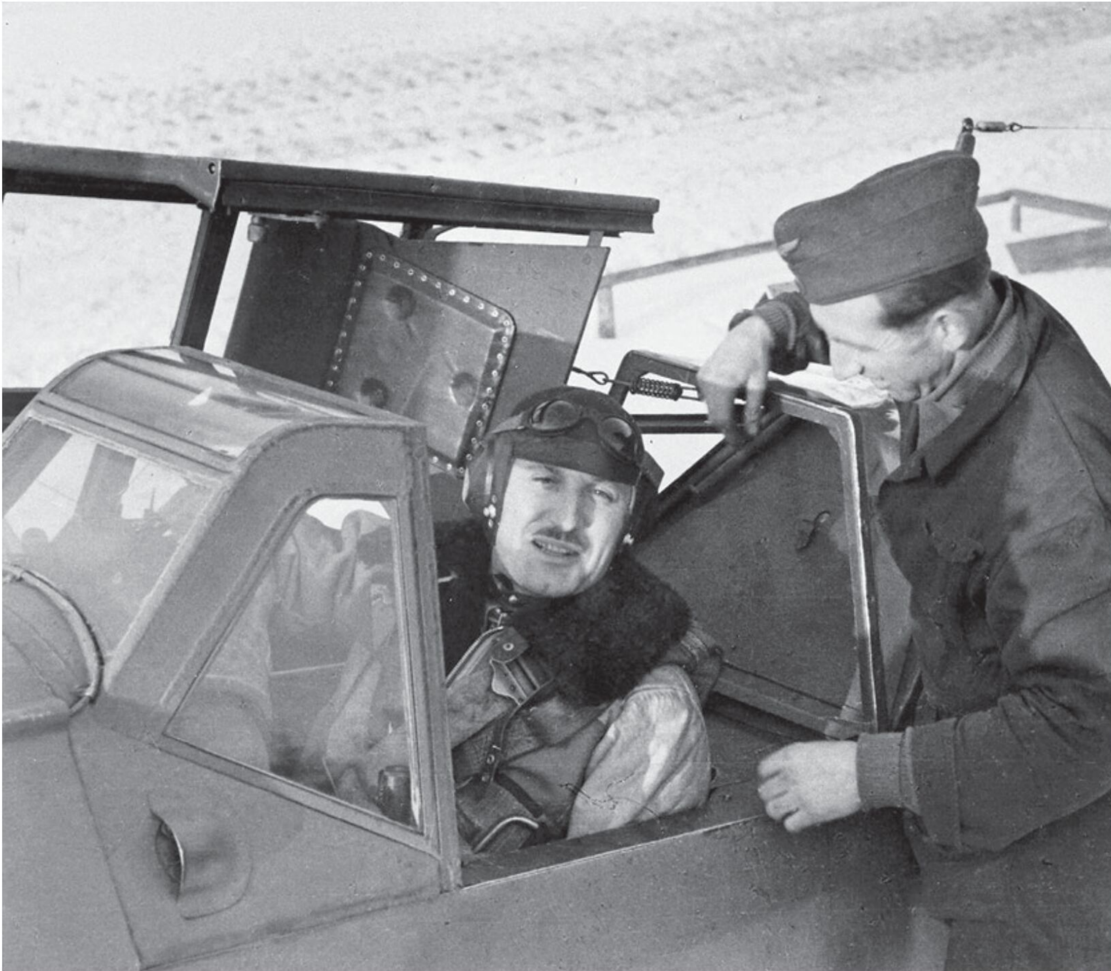
A mechanic assists Walter Dahl to strap himself into the cockpit of his Bf 109 G. Note the armor plate, which protected the pilot's head from fire from the rear, and the yellow octane triangle just forward of the fuselage Balkenkreuz (cross). (Photo courtesy of EN Archive collection)
