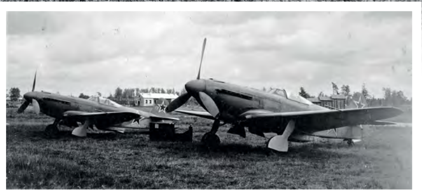
Powered by a Klimov VK-107A engine, the Yak-9U was the most advanced version of the fighter produced during World War Two.
