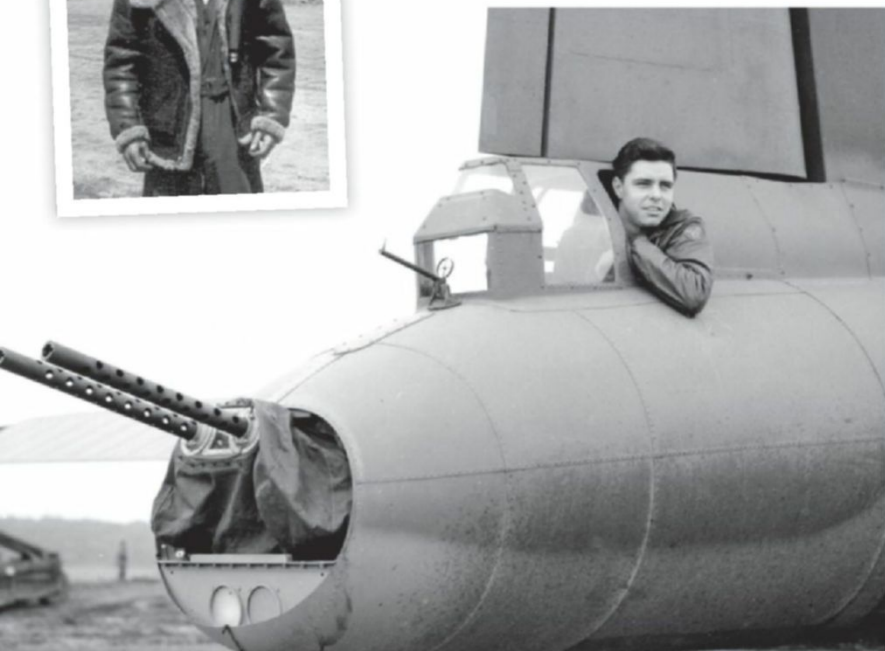
Above: Tail gunners' position stayed unchanged from the E- through late F-models when the Cheyenne Mod Center improvement came into the production line. (Photo courtesy of Stan Piet)
