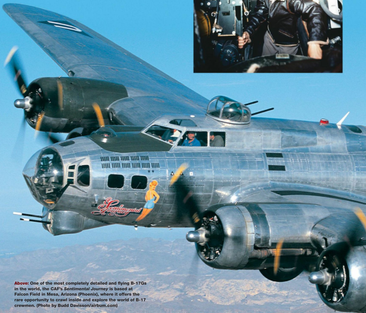
Inset: Access to the nose section of the Fortress for the navigator and bombardier/gunner was between the pilots raised seats. Emergency egress was available through the forward port side entrance hatch. (Photo courtesy of Stan Piet)
