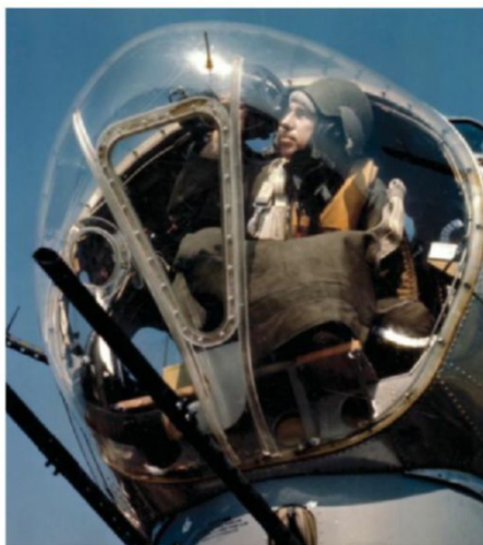
Left: Field mod twin-fifties in a B-17F to thwart head-on attacks. Center: The G-model Bendix chin along with the cheek gun addition in the Block-60 model gave the Fortress excellent head-on protection. (Photos by Stan Piet) Right: Norden bombsight, one of WW II's most tightly held secrets. (Photo by Heath Moffatt)
