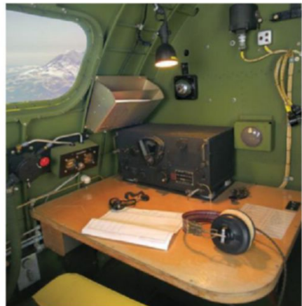
Left: The navigator's table behind the bombardier in the nose. (Photo by Heath Moffatt) Center: Navigators were provided with a cramped area in the nose along with a small roof astrodome for sighting work. (Photo courtesy of Stan Piet) Right: The radio operator's compartment with a small view to other 17s, flak bursts and scenery. (Photo by Heath Moffatt)
