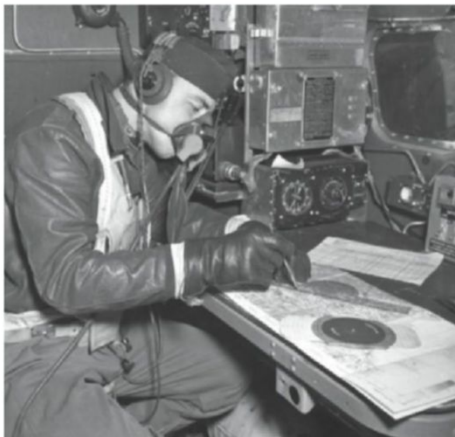
Left: The navigator's table behind the bombardier in the nose. (Photo by Heath Moffatt) Center: Navigators were provided with a cramped area in the nose along with a small roof astrodome for sighting work. (Photo courtesy of Stan Piet) Right: The radio operator's compartment with a small view to other 17s, flak bursts and scenery. (Photo by Heath Moffatt)
