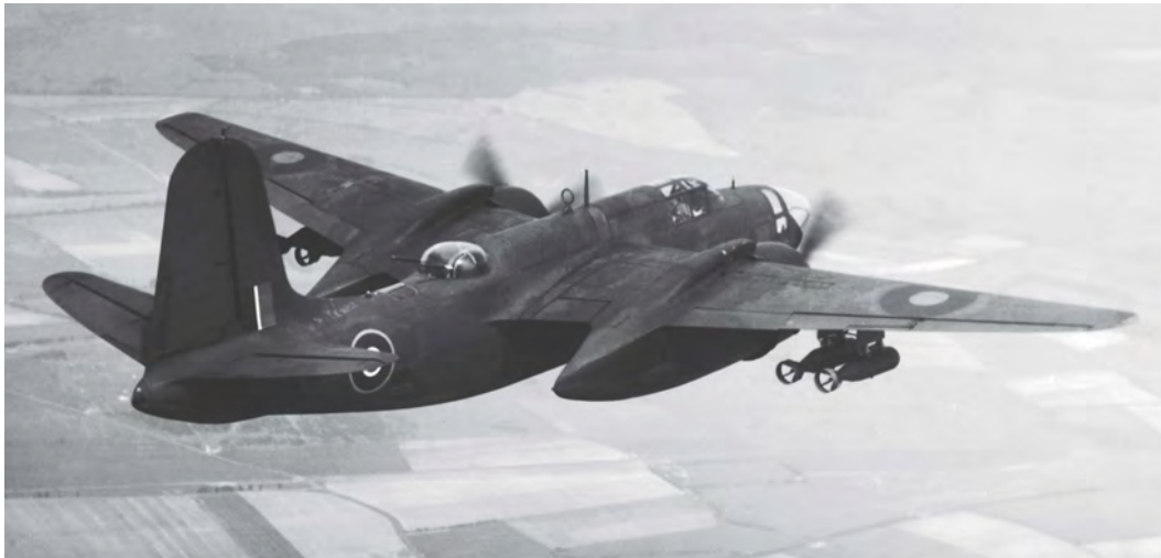
ABOVE: A bomb-toting Boston IV on a test flight over the UK. This variant was equivalent to the AAF's A-20J, itself an A-20G with a Plexiglas nose. KEY COLLECTION
