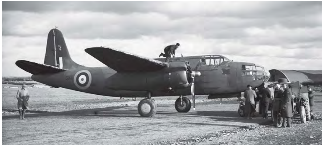
ABOVE: Boston I BD111 was among the aircraft diverted to the RAF from French orders. It was later converted into a Havoc I. AEROPLANE
