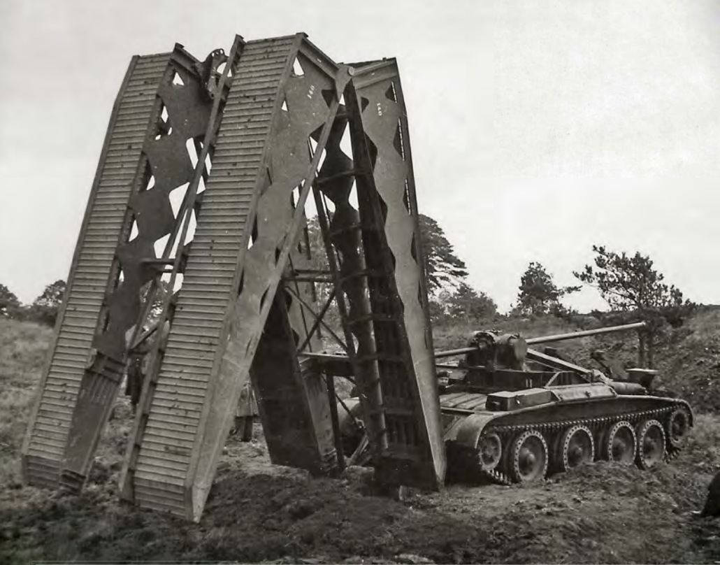
A Covenanter Bridgelayer on a training exercise in Britain with the threaded rod showing up clearly.
