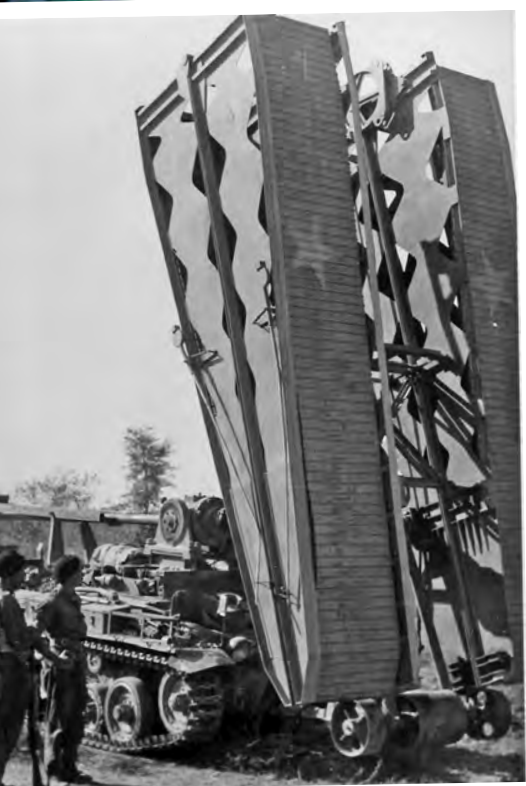
Above: A Valentine Bridgelayer in Burma attracts an audience as it goes through the laying process. Right: A Covenanter Scissors Bridgelayer serving with the 2/4th Australian Armoured Regiment bridges a stream on Bouganville in July 1945.
