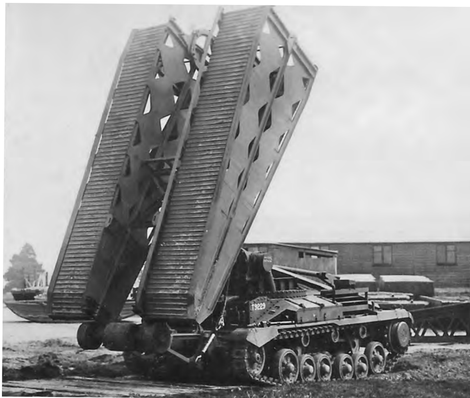
Above: A10 with the bridge at roughly the same angle. Notice how, with all the weight shifted to the front it pushes the nose of the tank down. Below: A10 viewed from behind, with the bridge nearly laid. The WD number is painted across the back so you can clearly see it, but notice how the threaded rod has moved through the gearbox.
