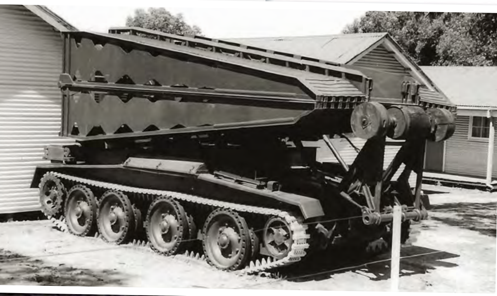
Above: The Covenanter Bridgelayer at Christchurch, showing how it hooked on to the bridge. Left: At the Australian Tank Museum in about 1970; the first Covenanter of any kind that I had seen.
