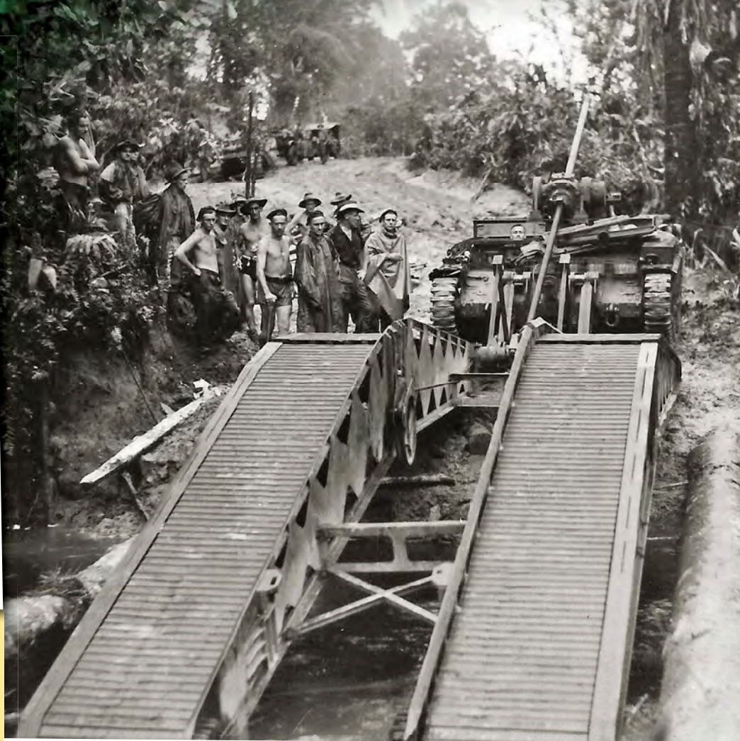
Above: A Valentine Bridgelayer in Burma attracts an audience as it goes through the laying process. Right: A Covenanter Scissors Bridgelayer serving with the 2/4th Australian Armoured Regiment bridges a stream on Bouganville in July 1945.
