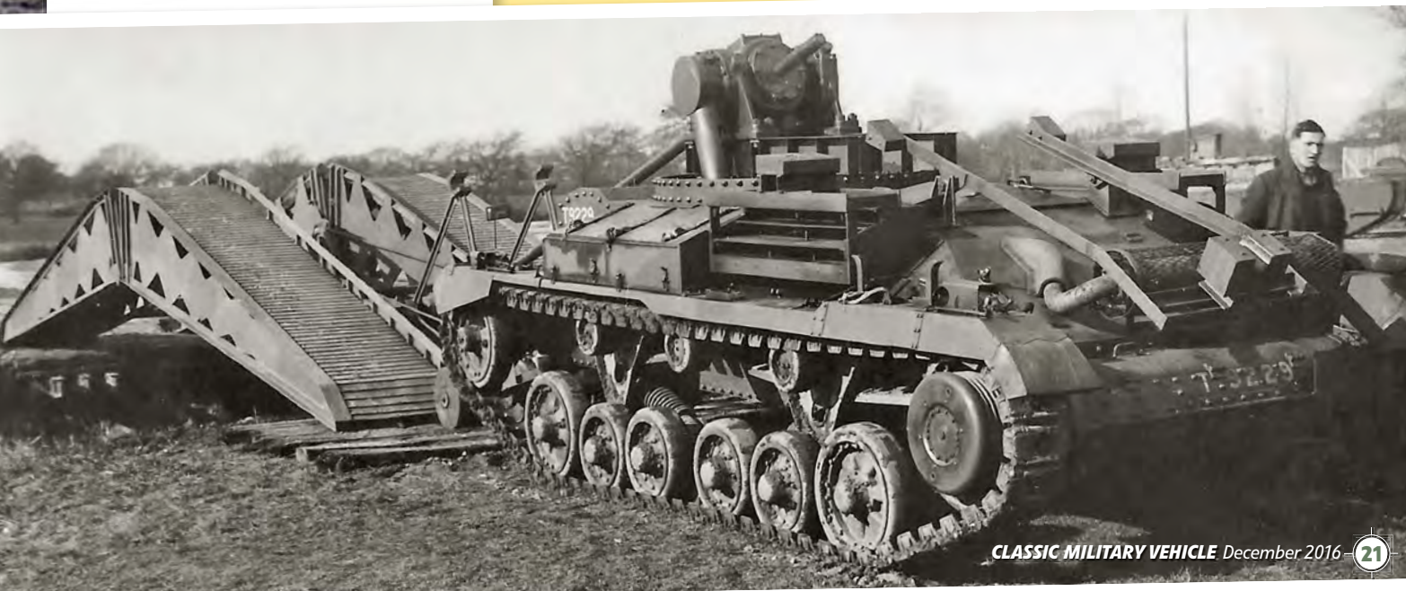
Above: A10 with the bridge at roughly the same angle. Notice how, with all the weight shifted to the front it pushes the nose of the tank down. Below: A10 viewed from behind, with the bridge nearly laid. The WD number is painted across the back so you can clearly see it, but notice how the threaded rod has moved through the gearbox.
