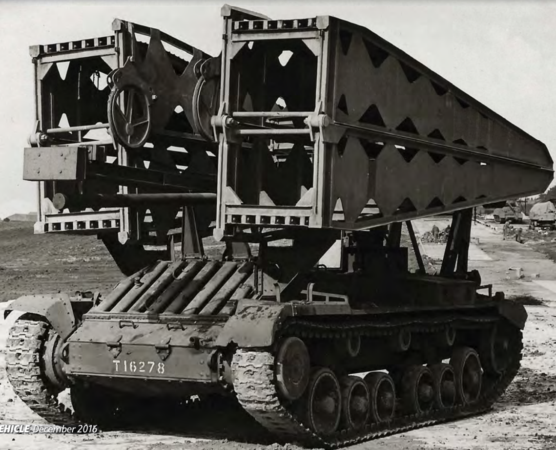
Above: Viewed from above, at the tower in Lulworth this bridgelayer is facing right but you get a good view of the threaded rod, running down the middle. Below: T16278 on a Mark 1 hull at Lulworth. This is said to be the pilot model of the Valentine Scissors Bridgelayer.
