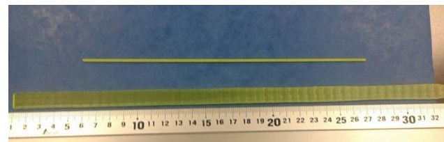
EFG-grown plate & fiber of LuAG:Ce from Adamant Namiki Co , Japan
