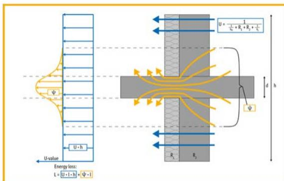
Fig. 1 Pattern of heat flow through a building enclosure with materials that allow lateral heat flow to a thermal bridge
