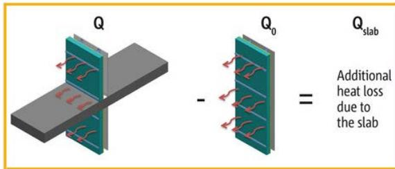
Fig.2 Example of process of determining the linear transmittance of a slab penetrating a wall
