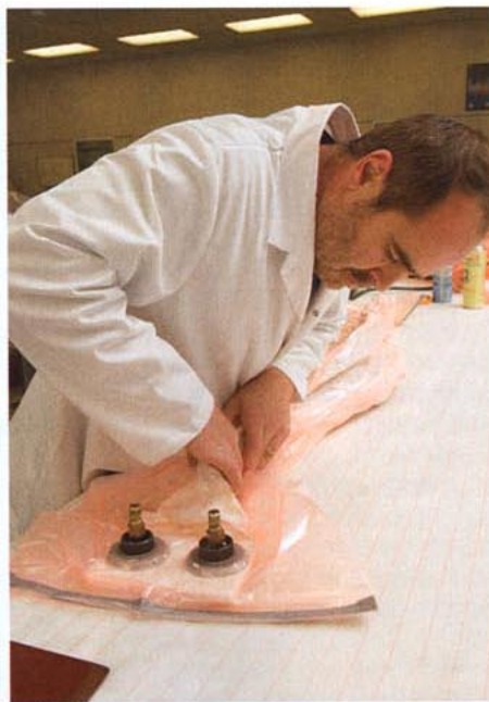
'Bagging up' before the wing spar goes into the autoclave: air passes through the 'breather blanket' (left) when the vacuum bag is being evacuated (right). The vacuum ensures that the temperature and pressure of the cure will be perfectly controlled
