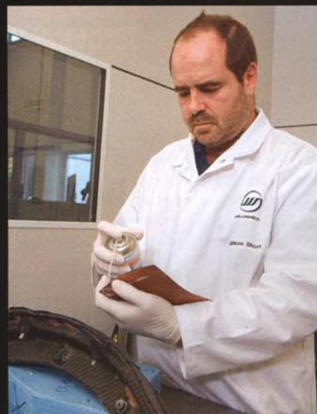
A wing spar starts out as many small sheets of carbon fibre, cut from a giant 50m roll and stuck into place on the mould
