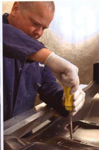
The two 'skins' of the 'mainplane' are trimmed and bonded (far left) then baked again to cure the adhesive. Then the various elements are screwed together to form the final assembly (above)
