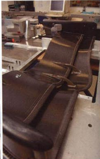
The two 'skins' of the 'mainplane' are trimmed and bonded (far left) then baked again to cure the adhesive. Then the various elements are screwed together to form the final assembly (above)
