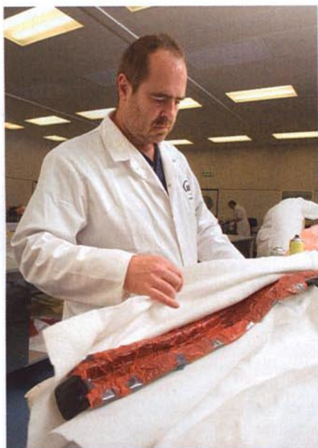
'Bagging up' before the wing spar goes into the autoclave: air passes through the 'breather blanket' (left) when the vacuum bag is being evacuated (right). The vacuum ensures that the temperature and pressure of the cure will be perfectly controlled
