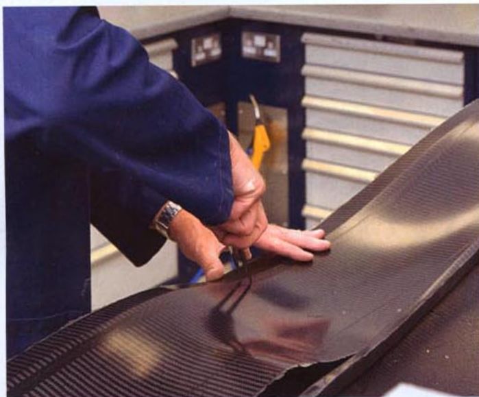
The two 'skins' of the 'mainplane' are trimmed and bonded (far left) then baked again to cure the adhesive. Then the various elements are screwed together to form the final assembly (above)
