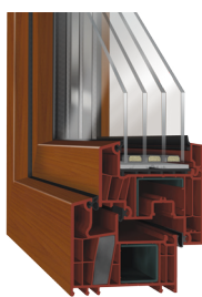
4-glass package 52 mm U_g 0,3 / \text{Wm}^2\text{K} spacer bar SWISSPACER Ultimate, krypton
