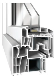
2-glass package 24 mm U_g 1,0 / \text{Wm}^2\text{K} spacer bar SWISSPACER V, argon
