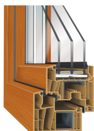
3-glass package 48 mm U_g 0,5 / \text{Wm}^2\text{K} spacer bar SWISSPACER V, argon
