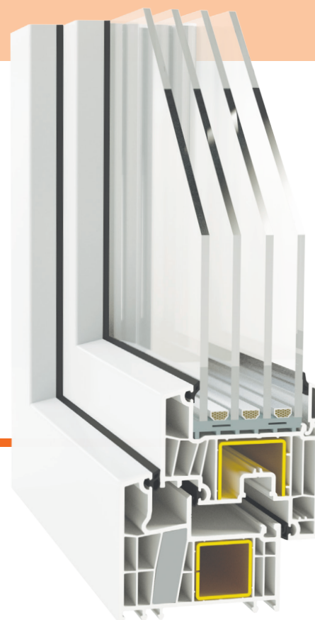
4-glass package 52 mm U_g 0,3 / \text{Wm}^2\text{K} spacer bar SWISSPACER Ultimate, krypton
