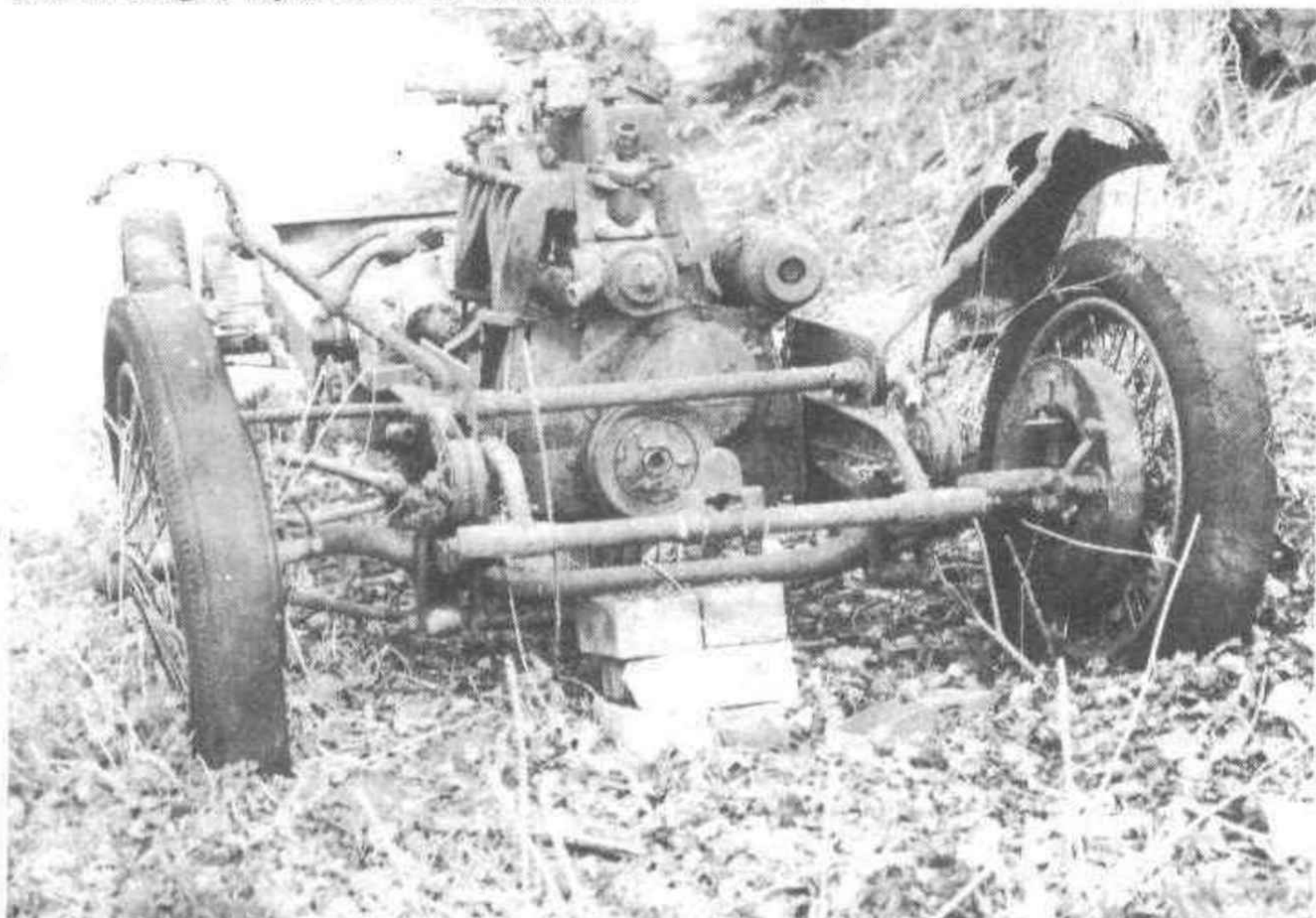
STILL THEY TURN UP. —This 1926 Type 40 Bugatti chassis, powered by a straight-six MG engine, has come to light in North Wales.
