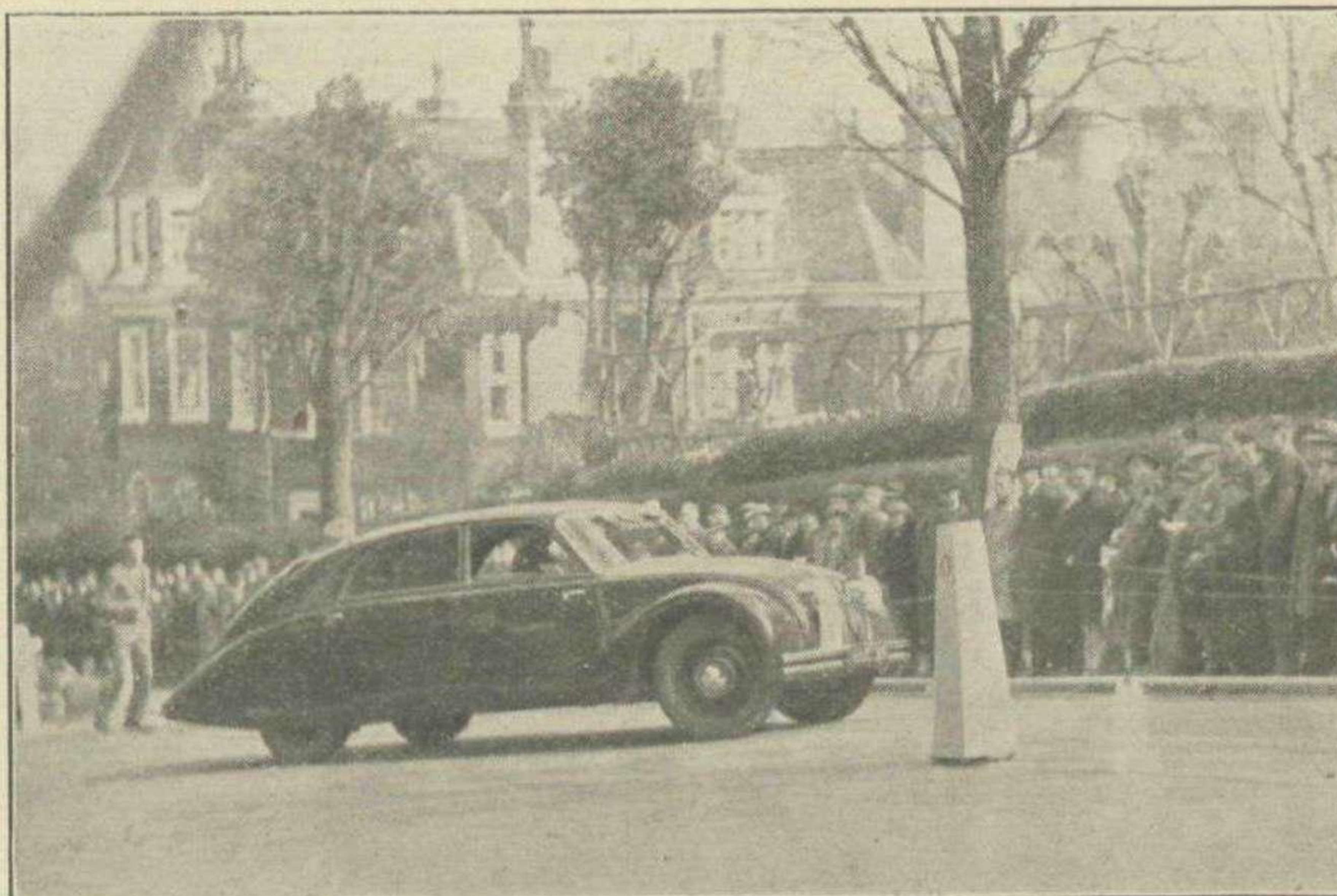
One of the most striking cars in the Rally was the airstream Tatra entered by C. W. Neville. The engine is at the rear and the car is scientifically streamlined.
