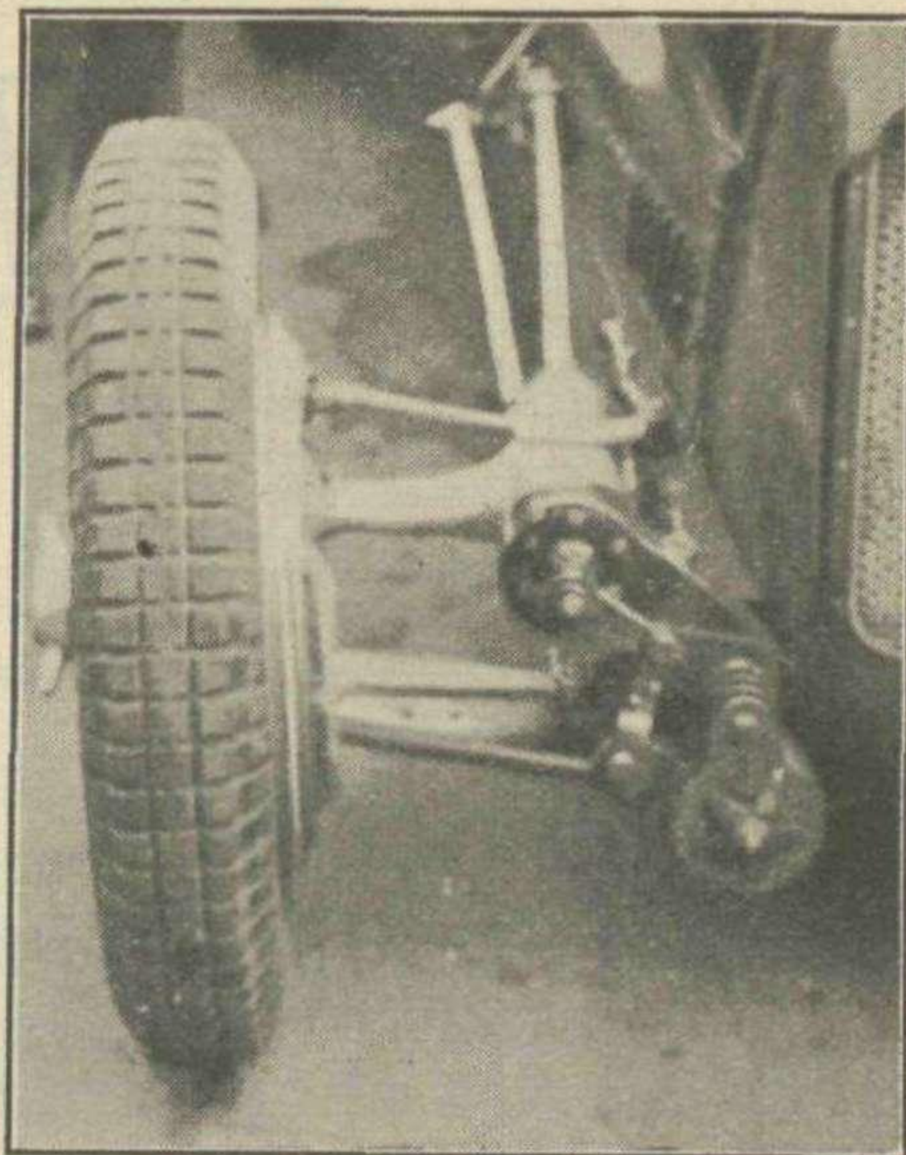
This is the Maserati system of torsion-bar suspension. The rod itself can be seen running parallel to the chassis frame, and above the steering rod. The shock absorber is connected up by means of a system of links.
