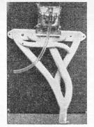
EXTRACTOR EXHAUST MANIFOLDS EXTRACTOR EXHAUST MANIFOLDS
