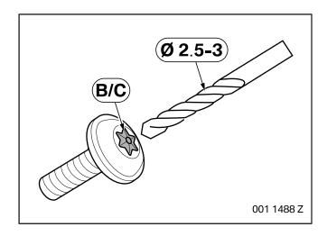
Extract the drilling chips during the drilling process.
