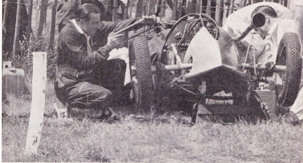
BRANDS HATCH: Don Gray, seeking more adhesion, applies a hacksaw to the tyres of his newly acquired Kieft.
