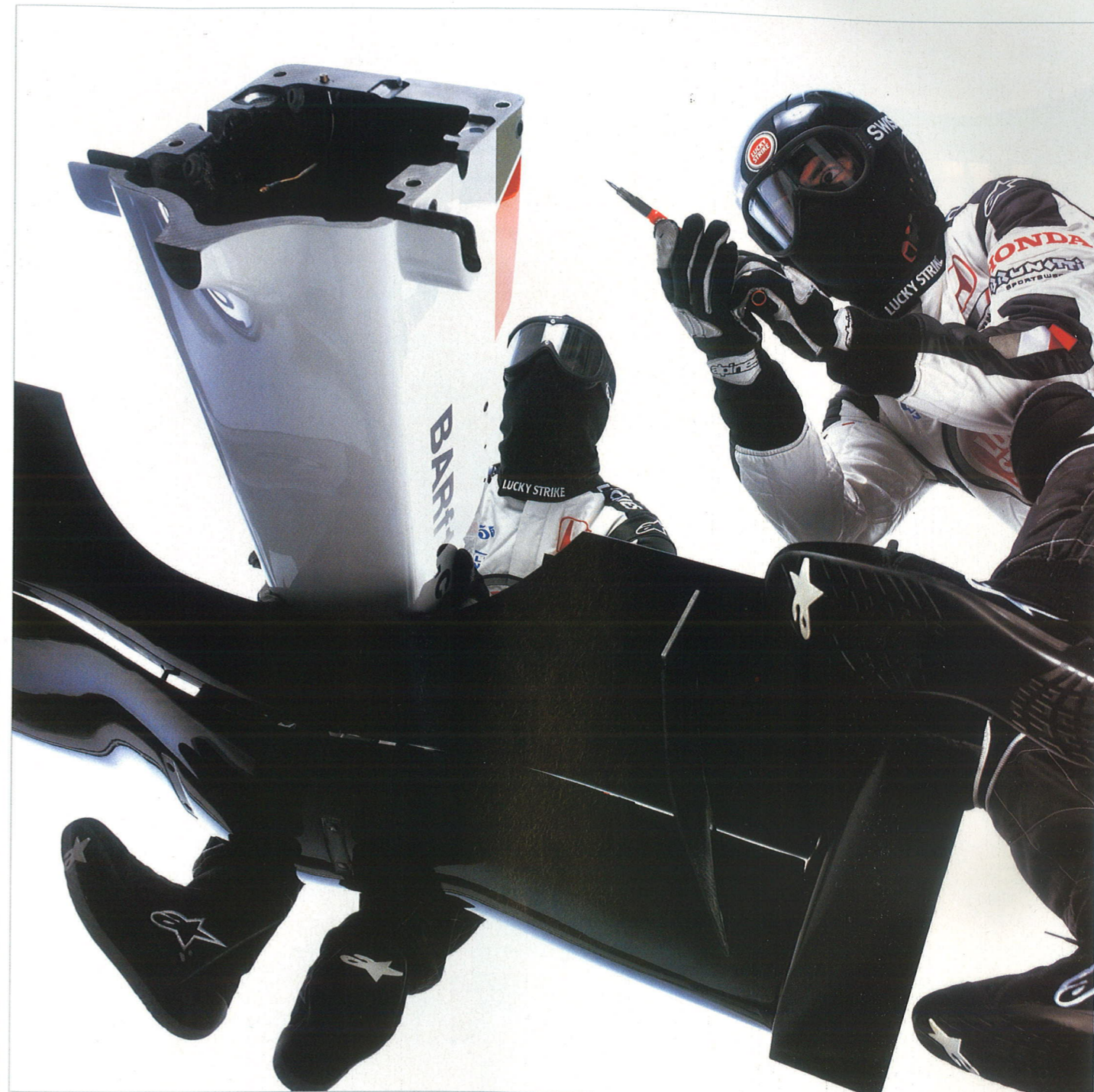
Equipment nose change keys, spare nose/wing, scissor jack, boots, personal fire extinguisher, helmet, goggles, overalls, gloves
