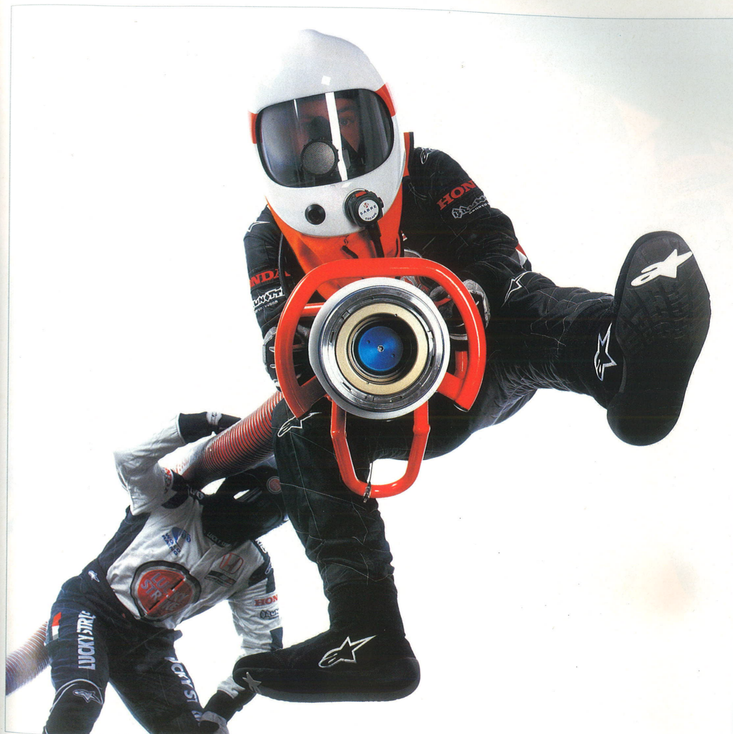
Equipment refuelling nozzle and hose, refuelling helmet, breathing apparatus, fire suit, boots, helmet, goggles, overalls, gloves
