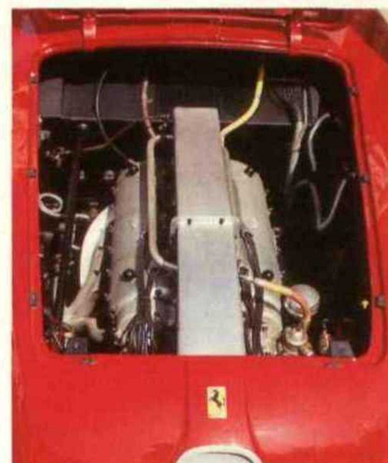
Tiny Colombo V12 puts out 118bhp
