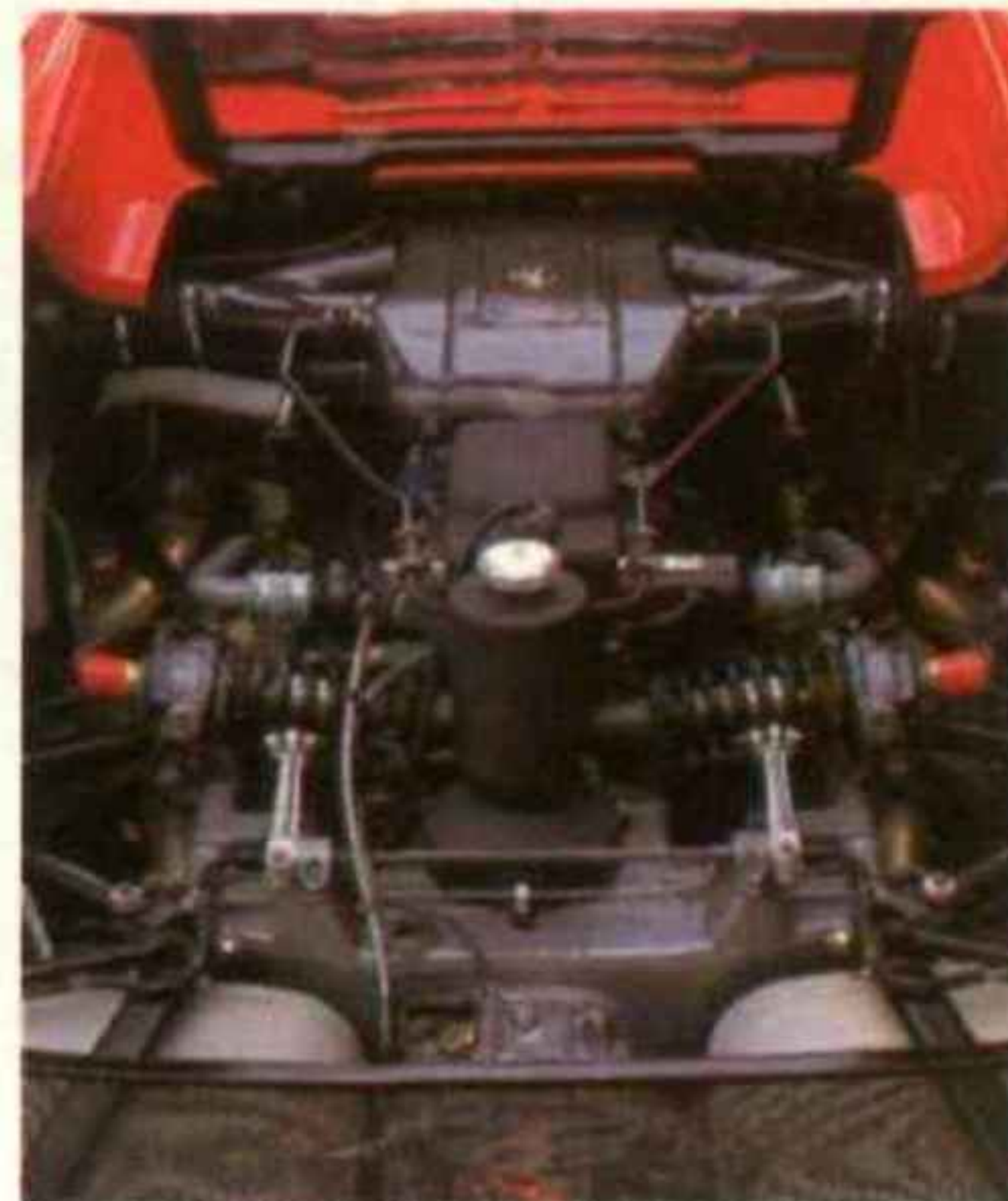
4.7-litre V12 has 60 valves, 513bhp
