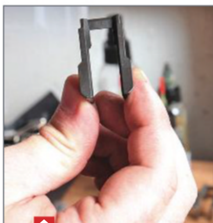
Polymer80's PF940C 80-Percent Compact Pistol Frame Kit comes with everything you need to complete the frame, including a red jig with instructions and the required drill bits. Once you drill the pinholes, remove the barrel block and smooth out the top, it's time to install Polymer80's rail modules. It's honestly easier to do than describe, but plenty of videos are available online.
