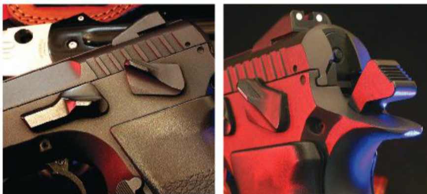
The Jericho 941 FS9's controls are all large and easy to operate, including the thumb safety and serrated hammer.
