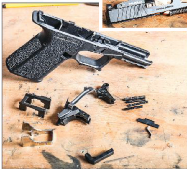
Completing the frame just requires a few extra parts, including pins, the fire control unit, the magazine release and the slide stop.
