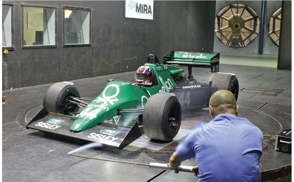
Here the front wing is at the maximum angle tested and the smoke plume shows the upwash at the trailing edge
