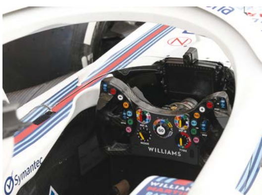
Williams bucks convention by being the only team to mount its dashboard on to the chassis rather than on the steering wheel
