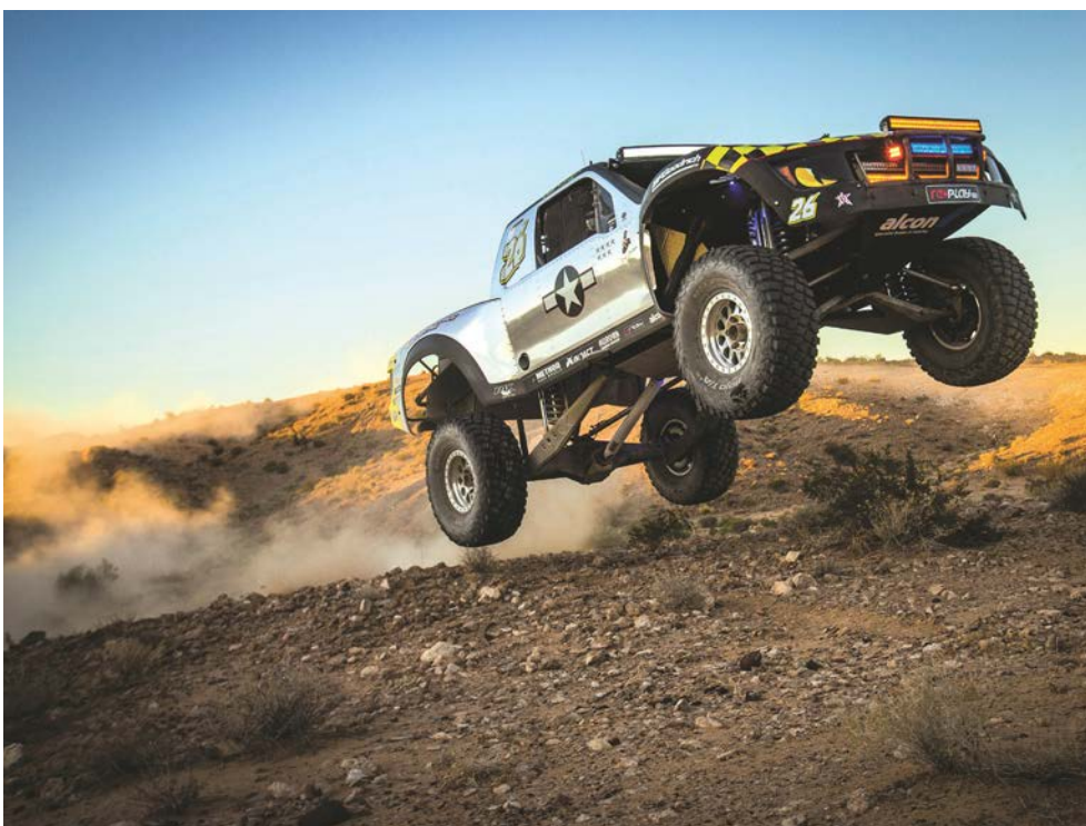
While 180cpm or even greater will suit racecars with proper downforce, off-road applications require much lower frequencies
