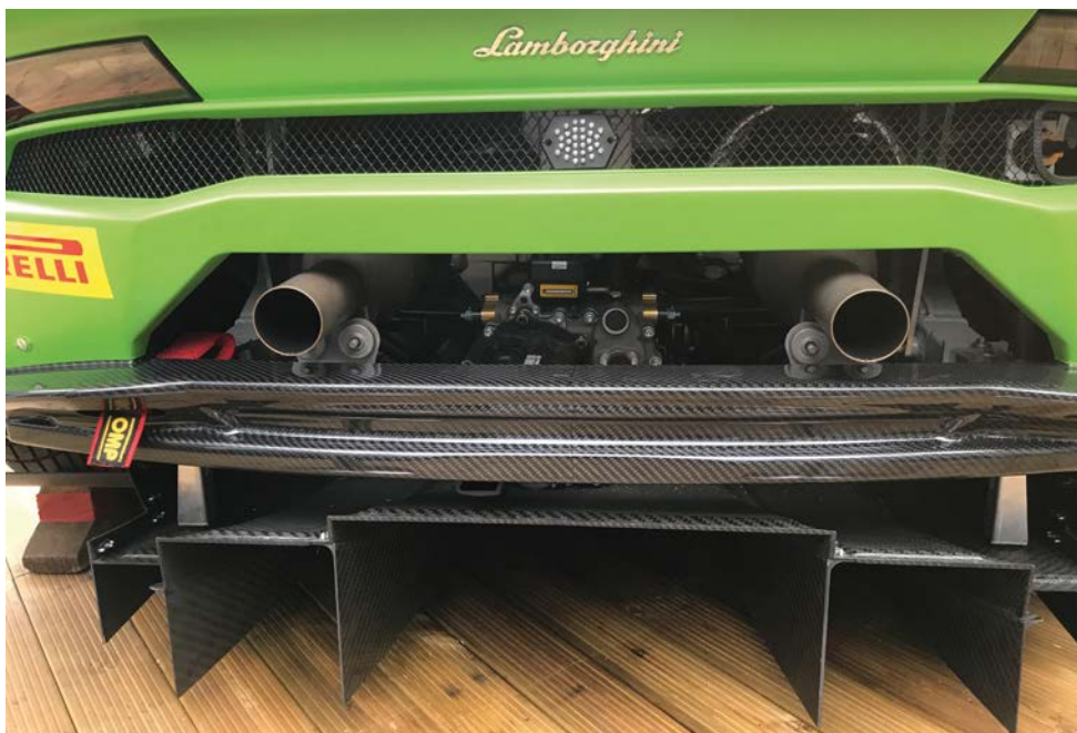
Lamborghini has improved the aerodynamics, albeit with a slight drag penalty. While there is little evidence of this work on the upper bodywork of the car, the underfloor has received plenty of attention. Note the Hor gearbox between the exhausts
