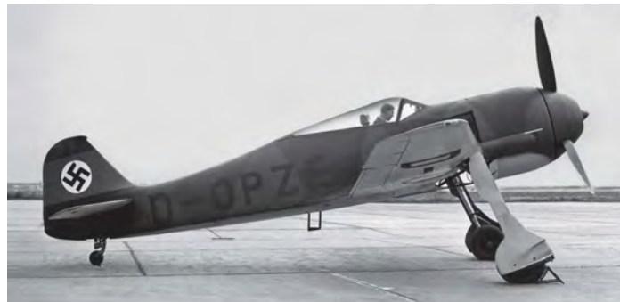
Although the ducted spinner on the first Fw 190 proved a failure, in almost every other way the engine design showed what could be done with a radial in an uncompromised fighter. VIA JAMES KIGHTLY
