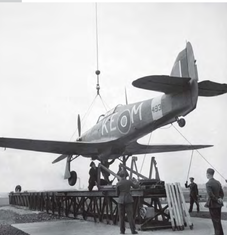
ABOVE: Sea Hurricane I Z4936 — originally built by Gloster — of the Merchant Ship Fighter Unit being readied for a launch from the training catapult located at Speke, Liverpool, with some of the firing rockets for the launch cradle leaning against the rear of the catapult assembly. 'KE' was the squadron code allocated to the RAF-controlled MSFU.
