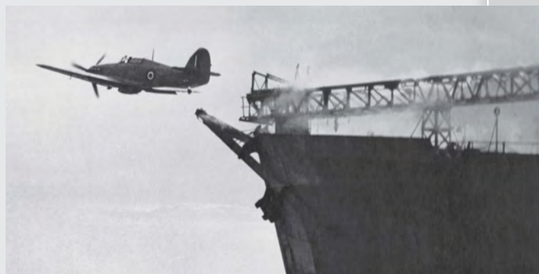
ABOVE: The 'one use only', catapult-equipped Sea Hurricanes launched from CAM ships, as here, were nicknamed 'Hurricats'.
