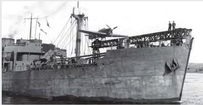
ABOVE: A 'Hurricat' on its launcher, ready to go. The flaps would be pre-selected in the take-off position.
