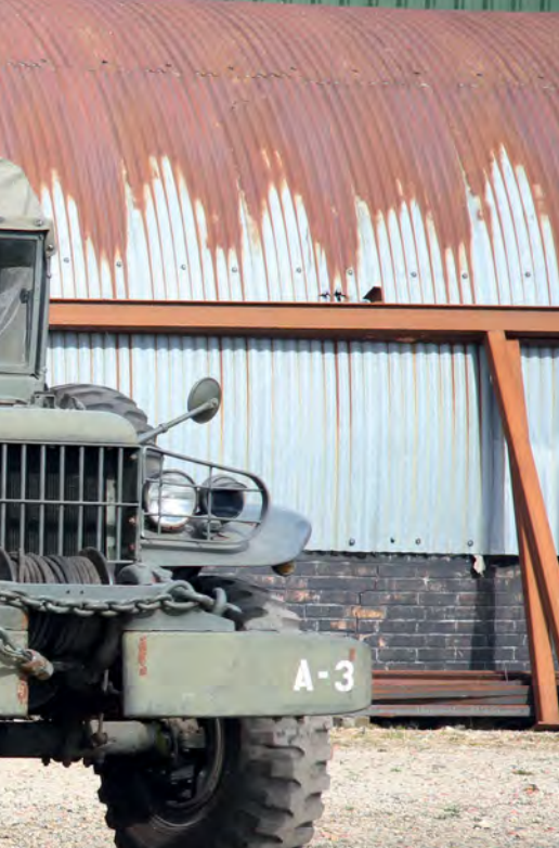
The three-quarter-ton WC series featured wider and lower proportions compared to previous models
