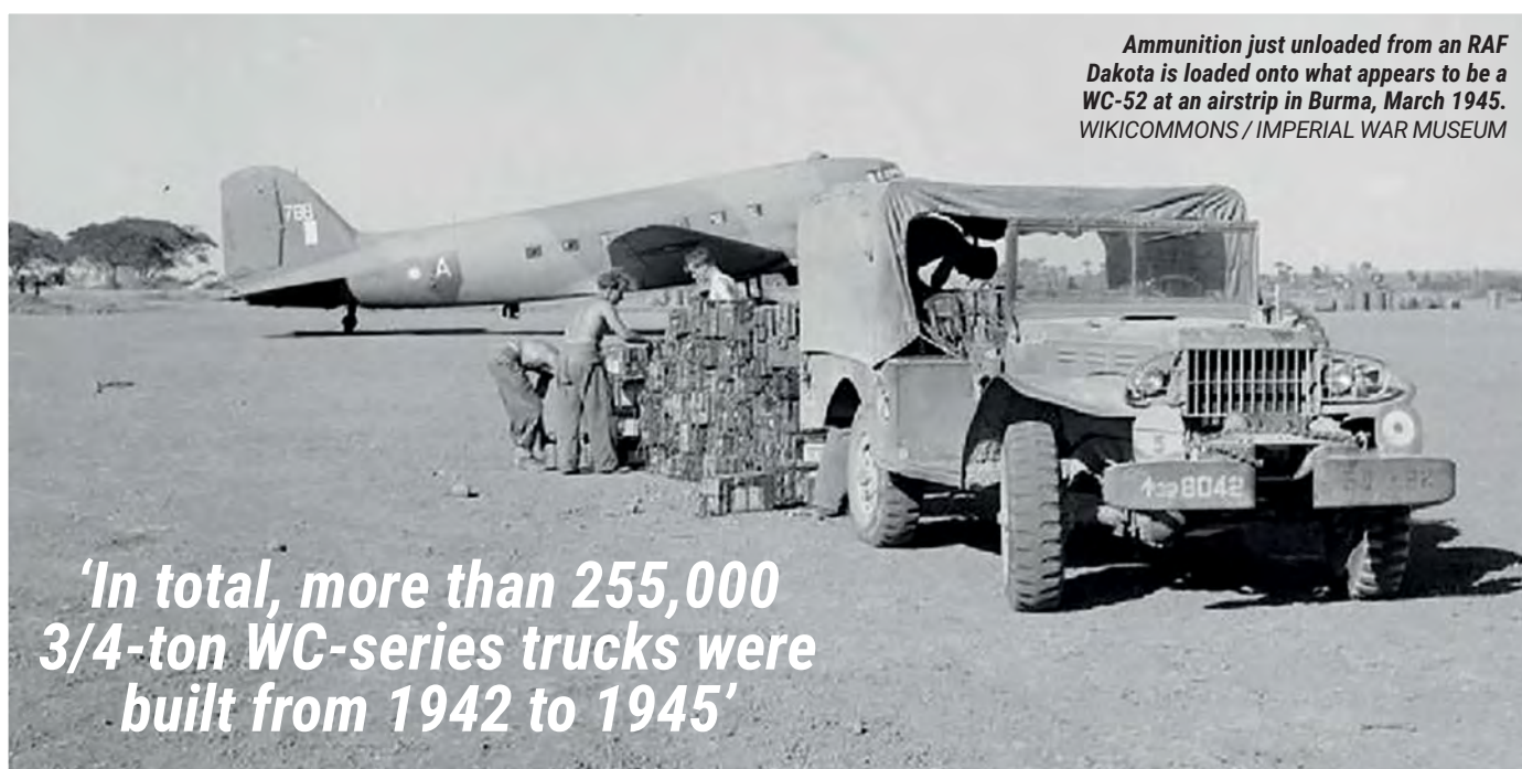
The three-quarter-ton WC series featured wider and lower proportions compared to previous models
