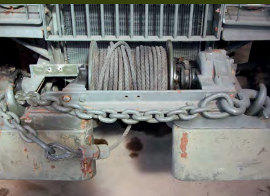
The WC-52 is differentiated from the WC-51 by the winch
