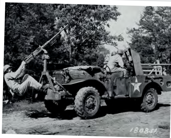
To increase firepower, a 50-cal. machine gun was mounted on the front of the M6 37mm GMC (June 1943). WIKICOMMONS / US ARMY
