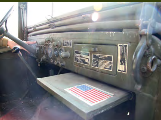
A map-reading board slides out from under the dash
