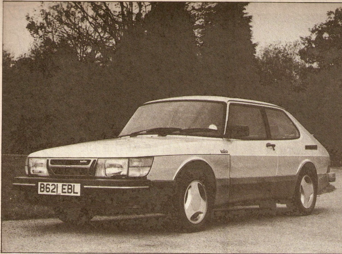
Deep front spoiler and side skirts make the Turbo 16S easily recognisable.
