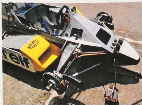
Renault RE30 in its new, «B» version has a lighter (by 4.5 kg) chassis, more effective aerodynamics (same downforce as with sliding skirts), revised suspension and a reliable 550 bhp (official). Weight will soon be down to the limit and there is electronic fuel injection to come later this year.
