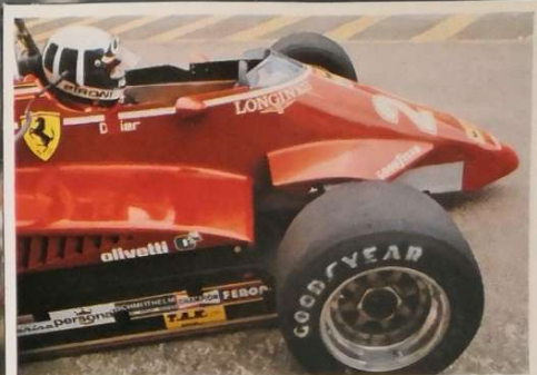
US-manufactured Goodyear tyres and a new honeycomb carbon fibre chassis designed by Dr Harvey Postlethwaite look like providing an answer to Ferrari's handling problems. Perhaps surprisingly, engines proved the team's downfall in SA: more development and a little less weight should make them winners in 1982.
