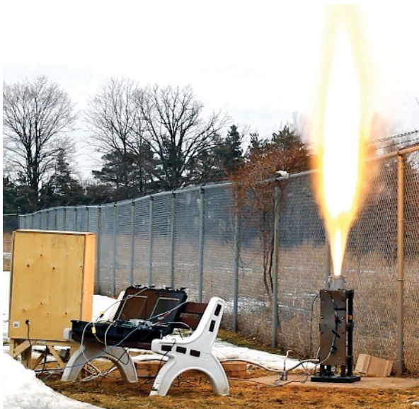
A still-frame taken from a static test fire of UTAT Rocketry's 2014-2015 hybrid rocket engine "Bia II". Powered by paraffin and nitrous oxide, this engine was designed to launch 10 lb payloads to 10,000 ft above ground level.
