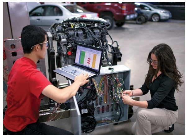
Ph.D. candidate Simon Wang and undergraduate Katy Hickey set up an open-architecture control system of engine combustion system development.
