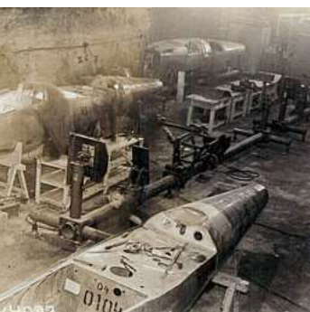
TOP: A row of rear fuselages awaiting components. Manufacturing delays were commonplace as essential parts took days to arrive where they were needed and regular powercuts caused blackouts underground.
