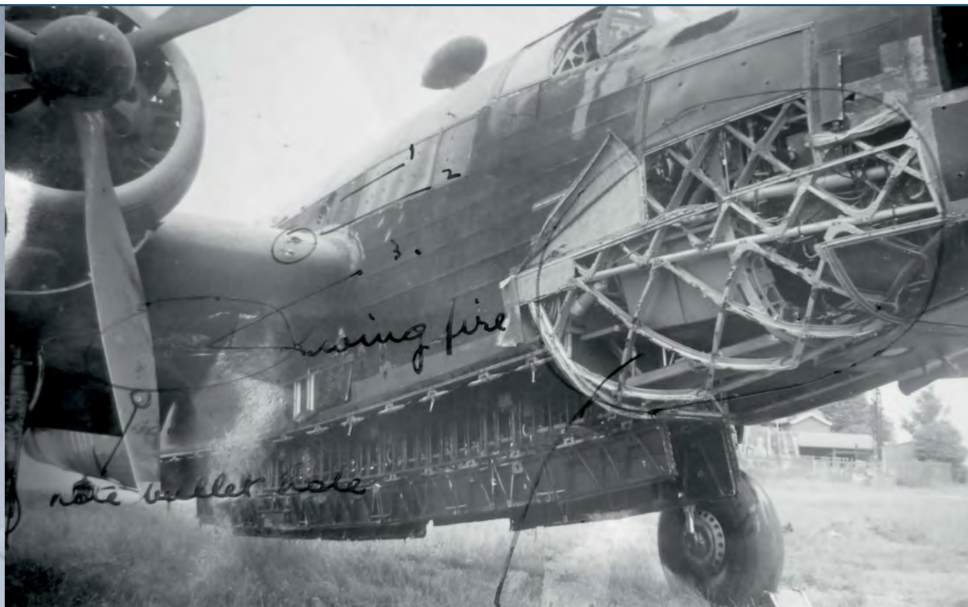
ABOVE: An annotated photograph of the damage Ward's Wellington received, also identifying the source of the second fire. (ANDREW THOMAS)
