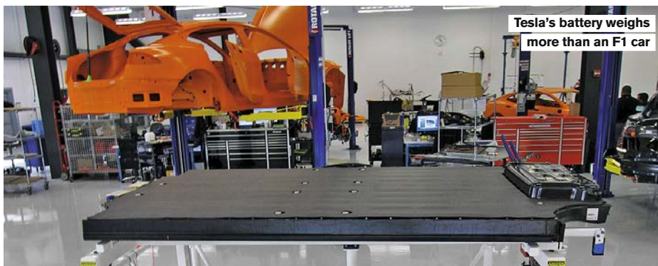
Tesla S road car uses over 7000 cells in its floor pan
