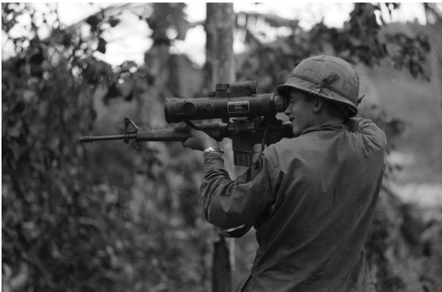
FIGURE 1 U.S. cavalry soldier poses with a AN/PVS-2 starlight scope mounted on an M-16 rifle, 13 Jan. 1967.
