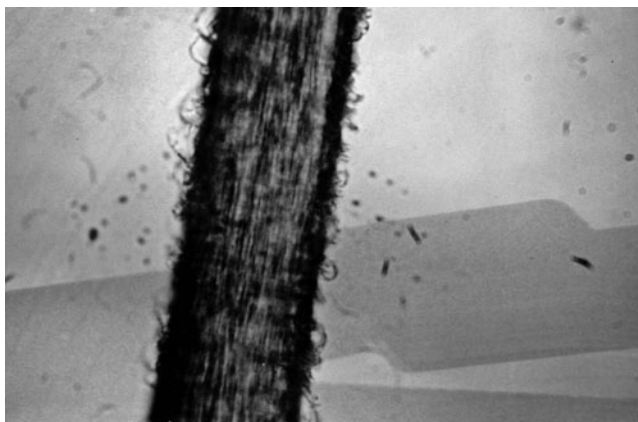
Fig. 4.4 Fiber was permanent waved on the head, after a few weeks cut, and treated with three alternating treatments of TEA lauryl sulfate and stearylalkonium chloride and observed in the light microscope. Note the lifted cuticle scales
