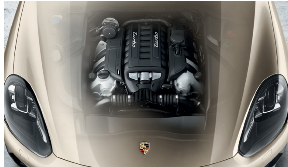
Cayenne Turbo: 553 lb.-ft. between 2,250 and 4,000 rpm, 520 hp at 6,000 rpm
