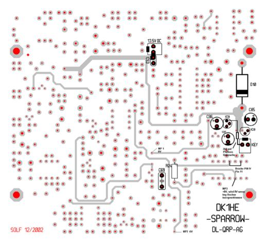
Section 1, Voltage regulation, keying section.
