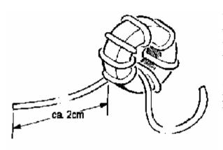
picture, e.g., has 8 turns. Well distributed means, that the wished number of turns fills about 270 degrees of the ring. That is about the maximum for toroids. If you are careful about this when you wind, you won't need to pull the turns apart later on, even though it to some degree is possible, turns shouldn't cross, but should be in one layer. Take care
