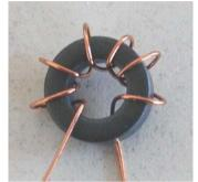
FT50-43 primary 4 turns isol. [ ] Tr.2 mounting wire, secondary 7 turns 0,5mm copper wire on the larger black toroid.
