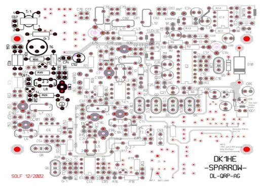
Section 7 Exciter and amplifier up to and including TR1/C86.
