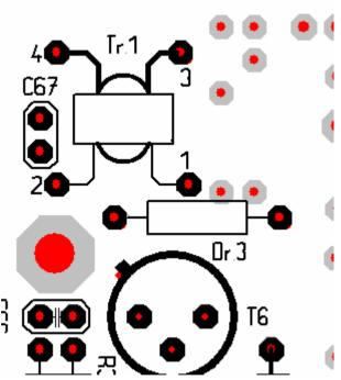
The transformer can be fitted. The secondary comes as 4/3, the primary as 2/1.
