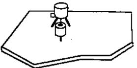
Ferrite bead placed over collector of T5
