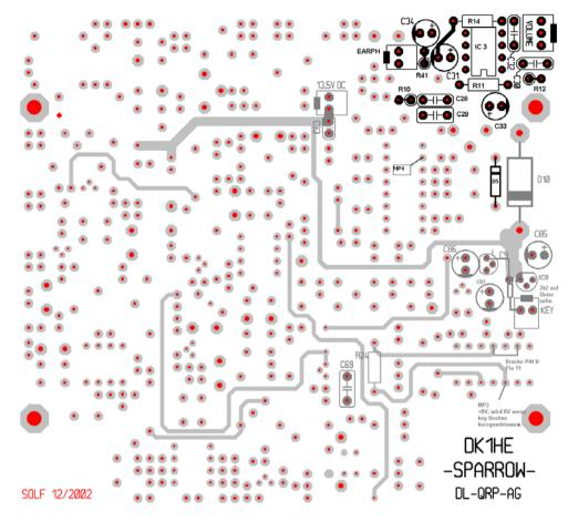
Section 2: AF output stage, AF preamplifier stage
