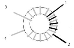
[ ] L8 toroid T37-2 red 20/5 turns 0,3mm copper wire reduce secondary windings if too much output
