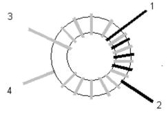
[ ] L6 toroid T37-2 red 20/7 turns copper wire 0,3mm
