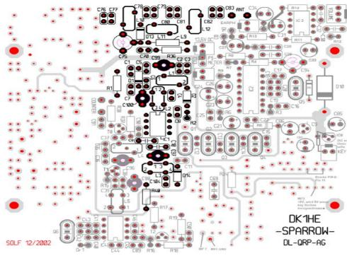
Section 5: RX input including Lowpass Filter LPF.
