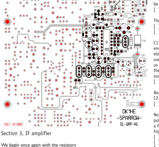
We begin once again with the resistors [ ] R3 220R [ ] R4 I8k R5 120R R6 2k2 R7 56k R8 27R [ ] R9 1k5 [ ] R13 470R Then follows a few capacitors of very high Q, the capacitors for the crystal filter. Here we use either ceramic capacitors or NPO multilayer capacitors. Here it is not a matter of temperature coefficient, but only the Q. [ ] C12 220pF NP0 ] C11 220pF NP0 C13 220pF NP0 [ ] C14 220pF NP0 C15 220pF NP0
